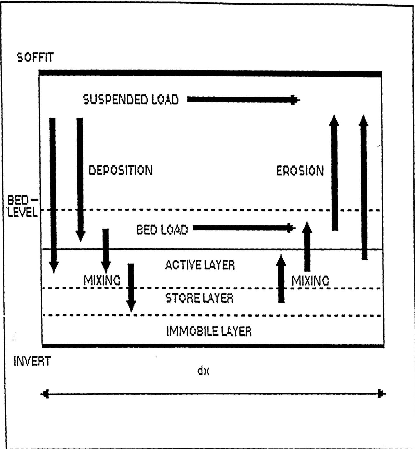
FIGURE 3 PROCESSES IN THE LINK SUBMODEL
