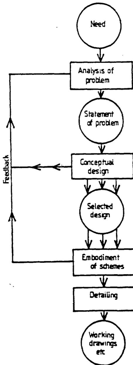
Figure 1. French's model of the design process.
