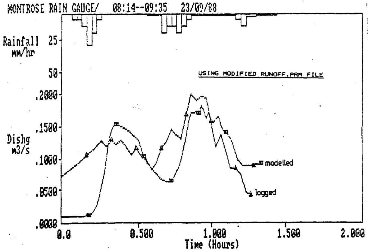
VERIFICATION EVENT 23/9/88 RECORDED/MODELLED FLOW AT GAUGE MANHOLE
