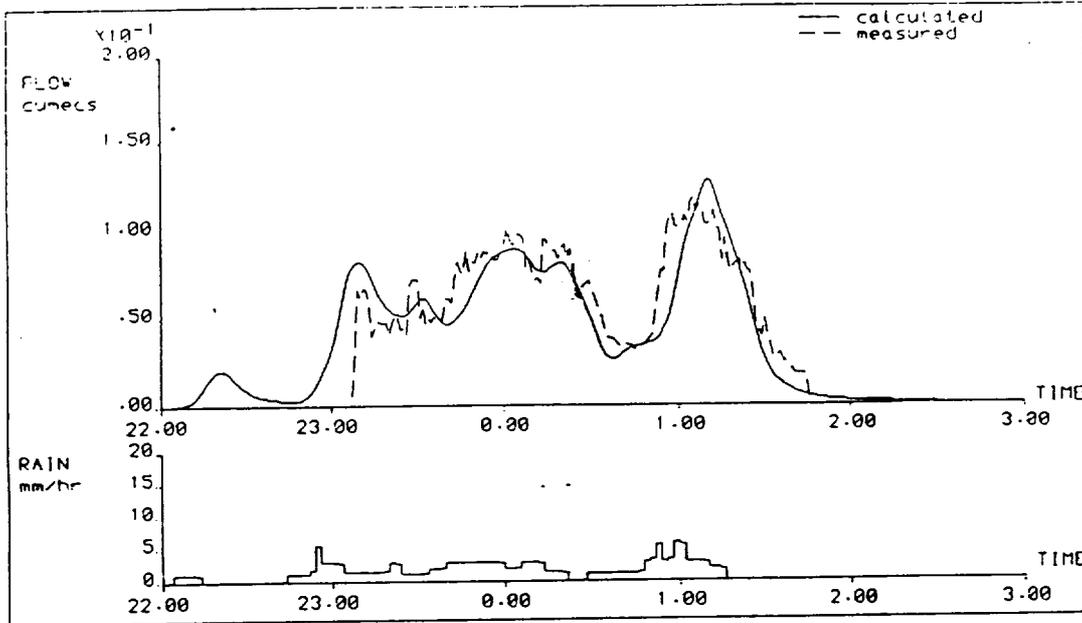
Figure 6 Comparison of WASSP prediction with measured flow at monitor site 2.
