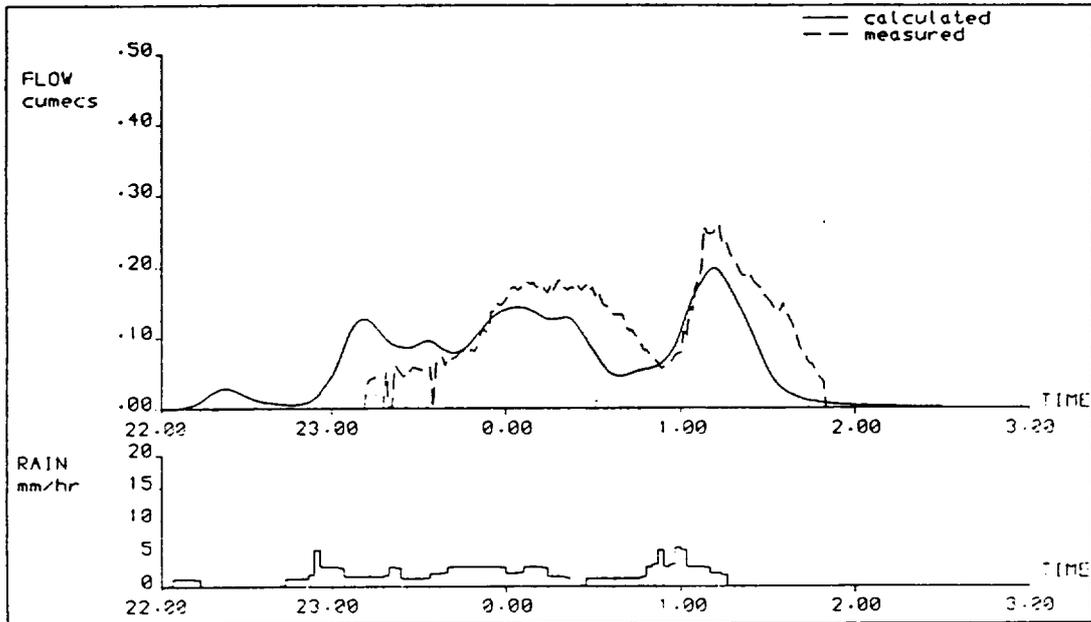
Figure 5 Comparison of WASSP prediction with measured flow at monitor site 1 (Bacon Lane Overflow).
