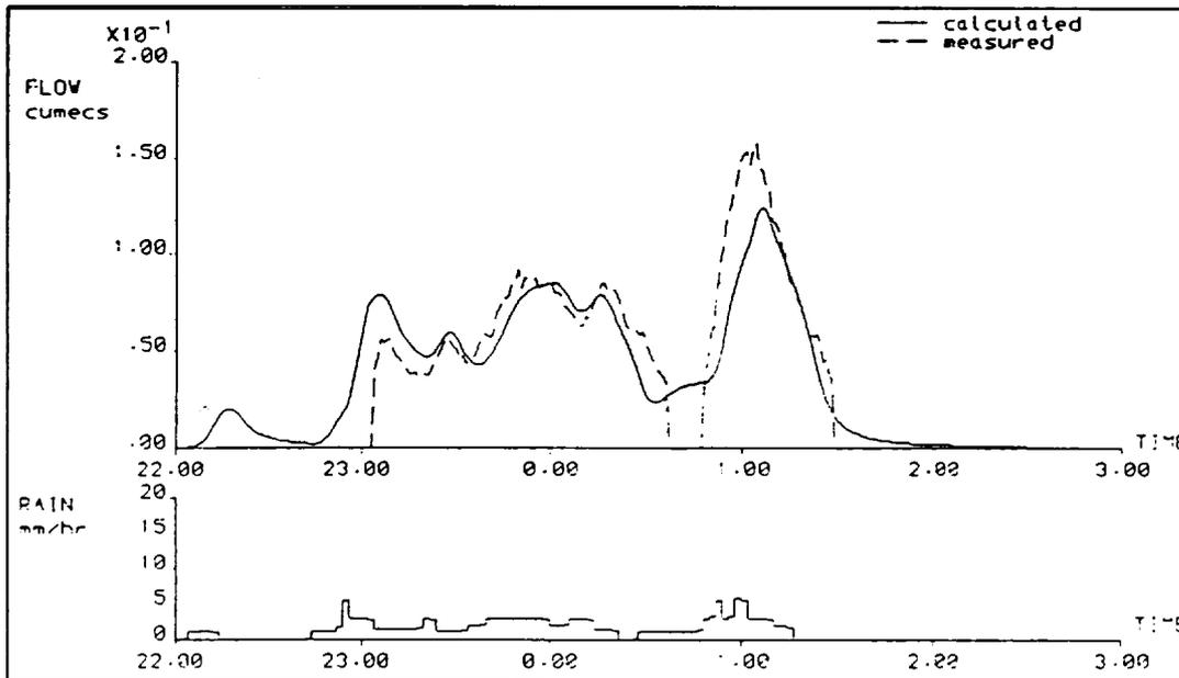
Figure 7 Comparison of WASSP prediction with measured flow at monitor site 3.
