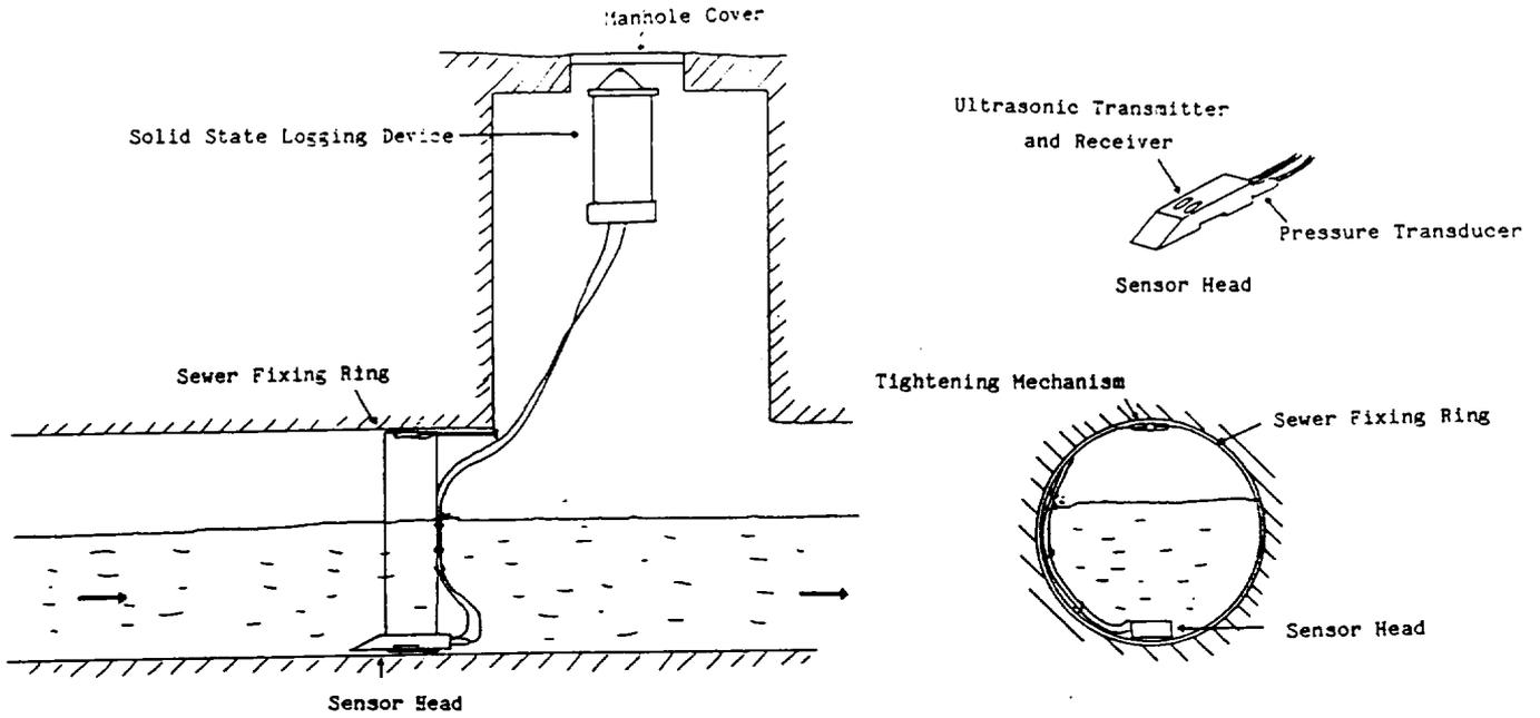
Figure 4 Typical Flow Survey Equipment Installation
