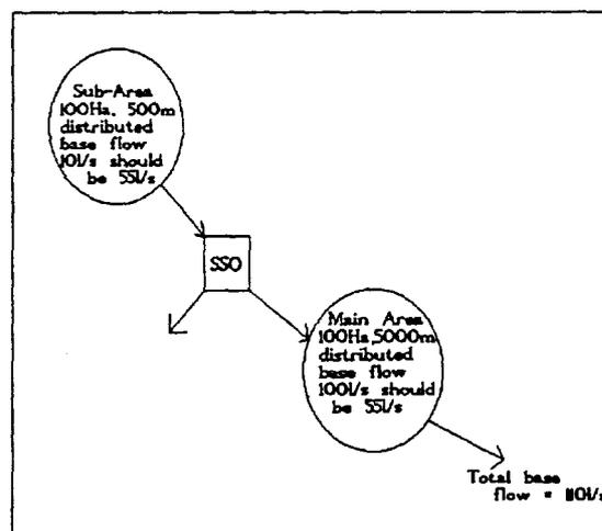
It is possible to get around this type of problem by carrying out a manual calculation and then attributing appropriate base flows to the pipes in the sub-area. There would still, however, be the drawback that the flows calculated would remain fixed for the duration of the simulation period. In reality, base flow can fluctuate considerably
