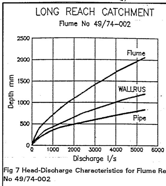
Fig 7 Head-Discharge Characteristics for Flume Ref No 49/74-002
