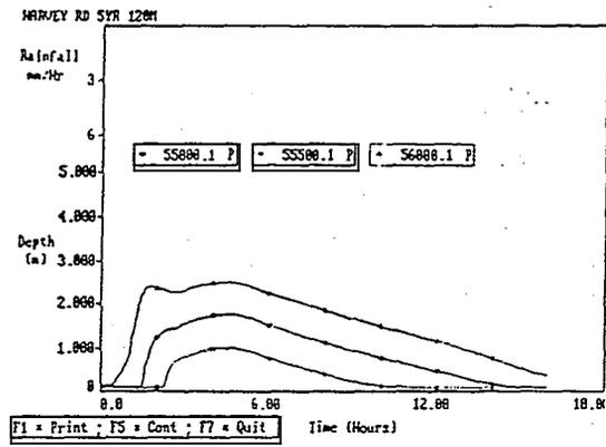
SPIDA has also proved to be particularly useful in the simulation of the performance of a number of low-side-weir CSOs on large diameter sewers, where spill commences before pipe-full conditions are reached and where the downstream surcharge is having a significant effect on the onset of spill.
