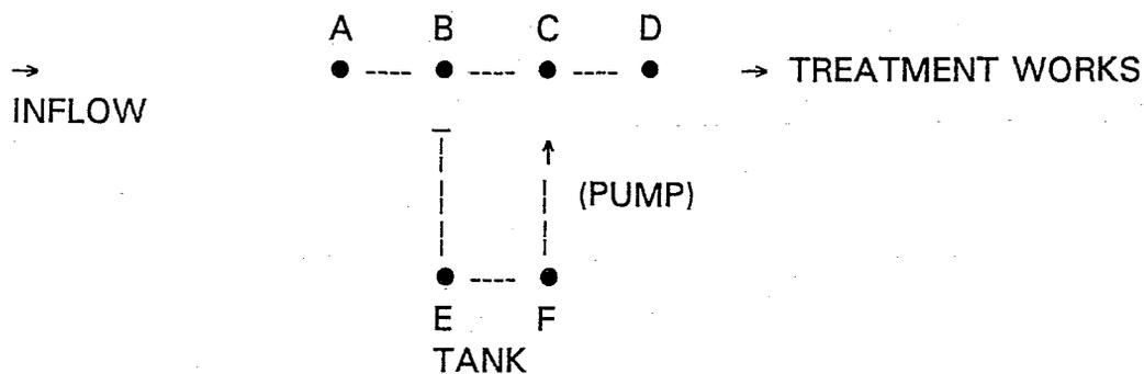
In the above system there is an inflow at A and an outfall at D. At point B we are able to divert flow to point E where there is a storage tank. The flow in A-B is continually monitored. When the flow in A-B reaches a set value, part of the flow is diverted into the storage tank at E. When the flow in A-B falls below a set value, the flow to the treatment works is maintained by increasing the return flow in F-C.
