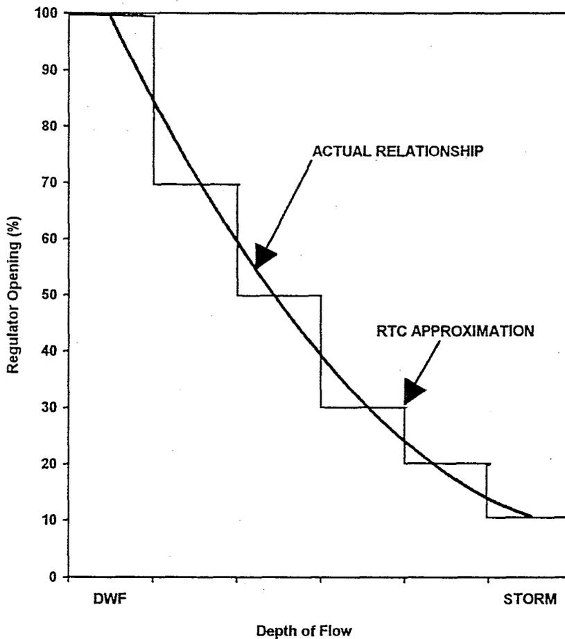
Figure 2. Definition of regulator mode of operation.
