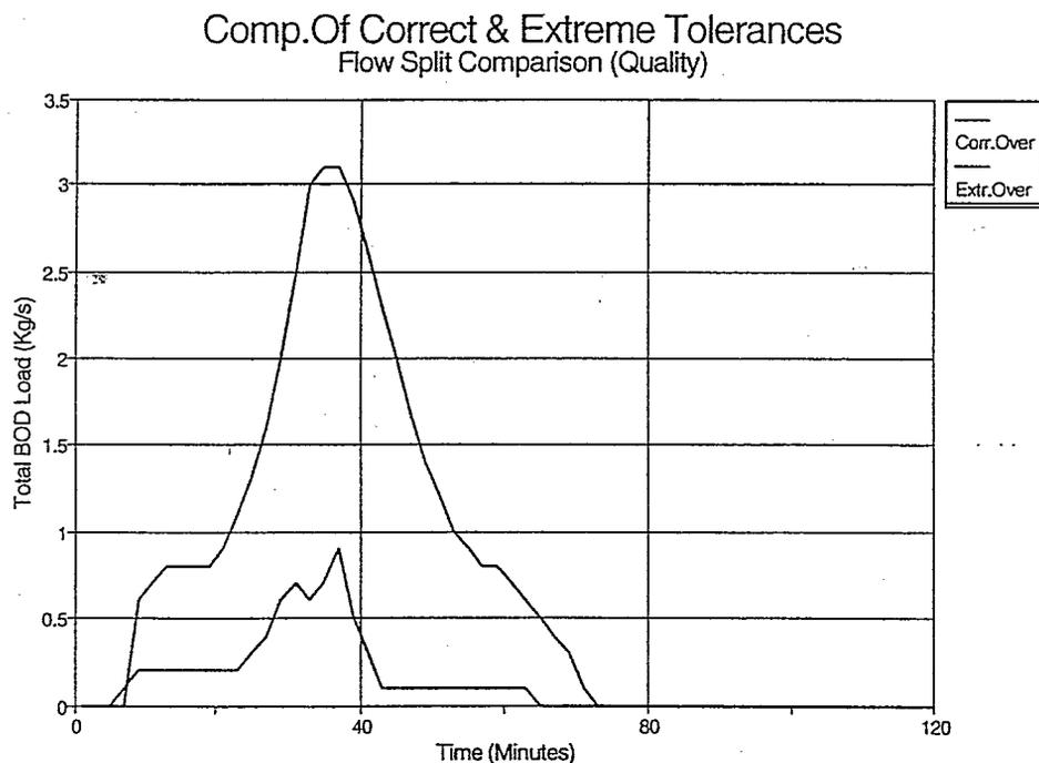
**Figure 6 : Overflow Spill Quality**
