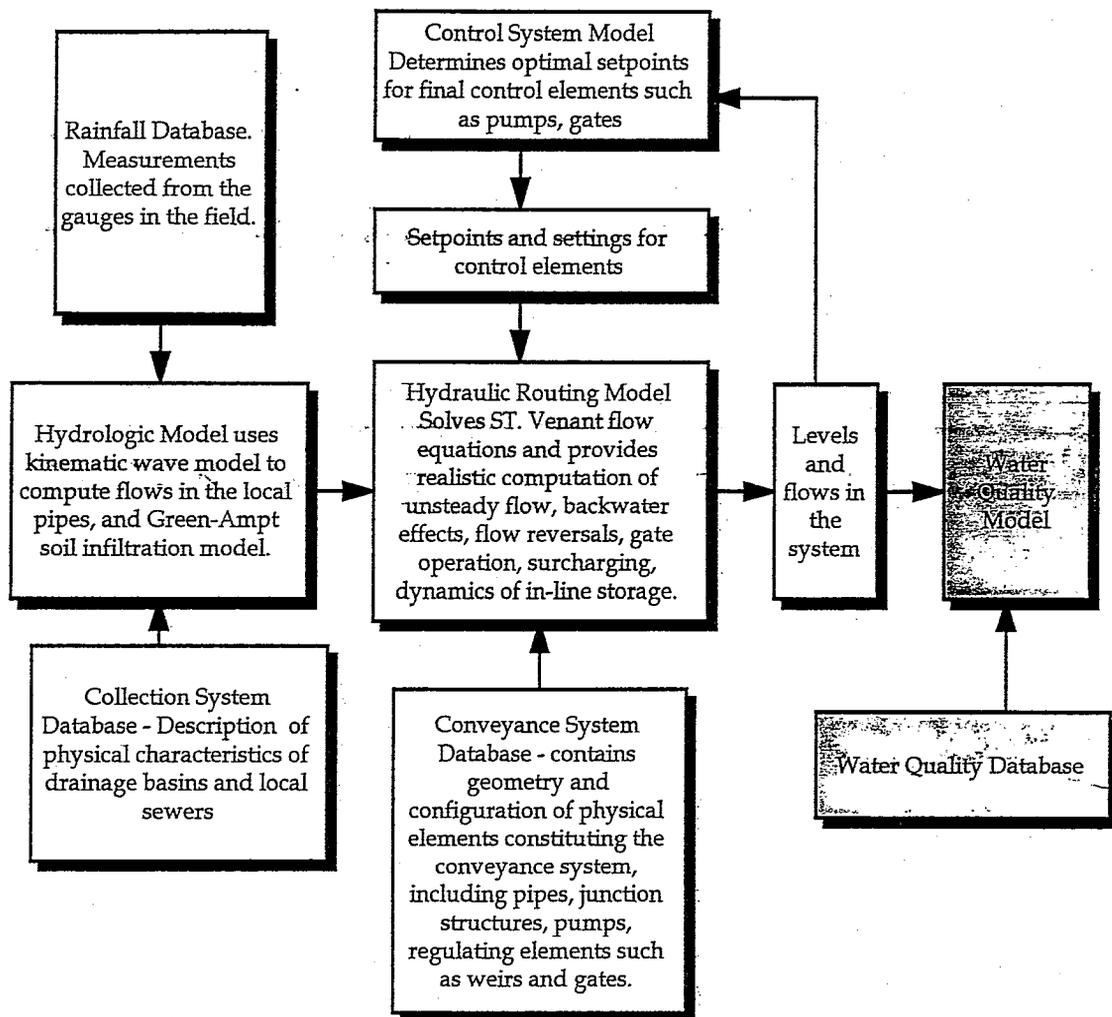
**Figure 2. Modelling system components**
