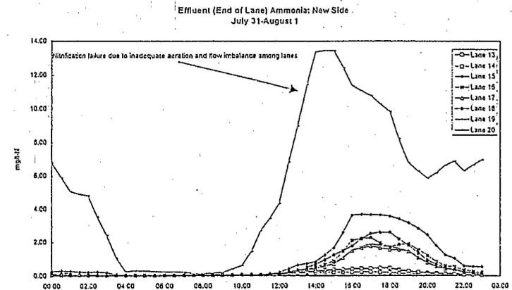
Figure 4: New Side - Effluent Ammonia Concentrations
