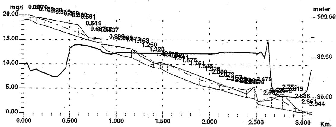
Once the river model had been calibrated the model was re-run by removing the CSO impacts from critical events one by one and determining the resulting reduction on impact on the river by comparison with the baseline impacts. Once this was done the CSO's could be ranked in terms of impact on the river.
