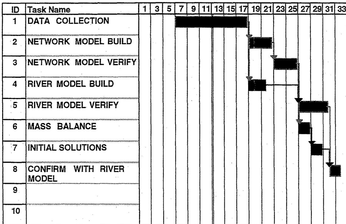
attempt to calibrate the river model for storm events. It is essential that the Environment Agency are in agreement with the calibration or verification of the network or the wastewater treatment works model. Because of the potential number of critical paths on the study, which may run through data collection in the network or river and through model build in the
