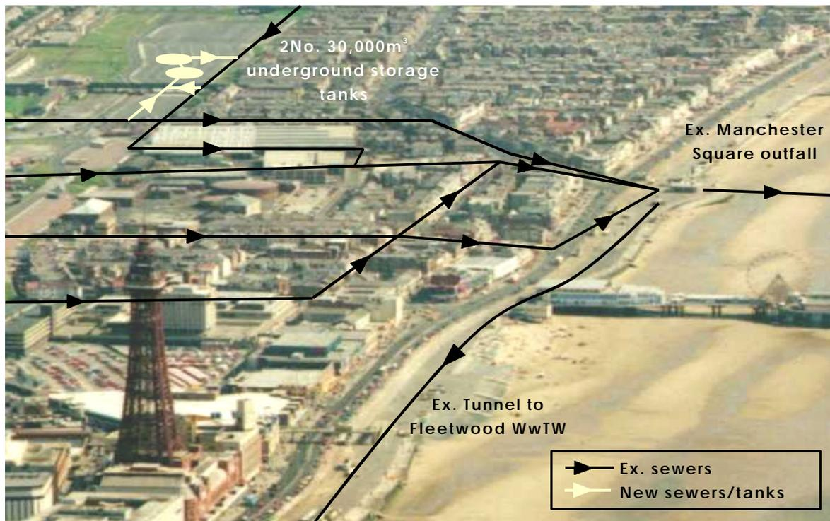
**Figure 8** : Aerial View of the Blackpool end of the Fylde Coast Tunnel
