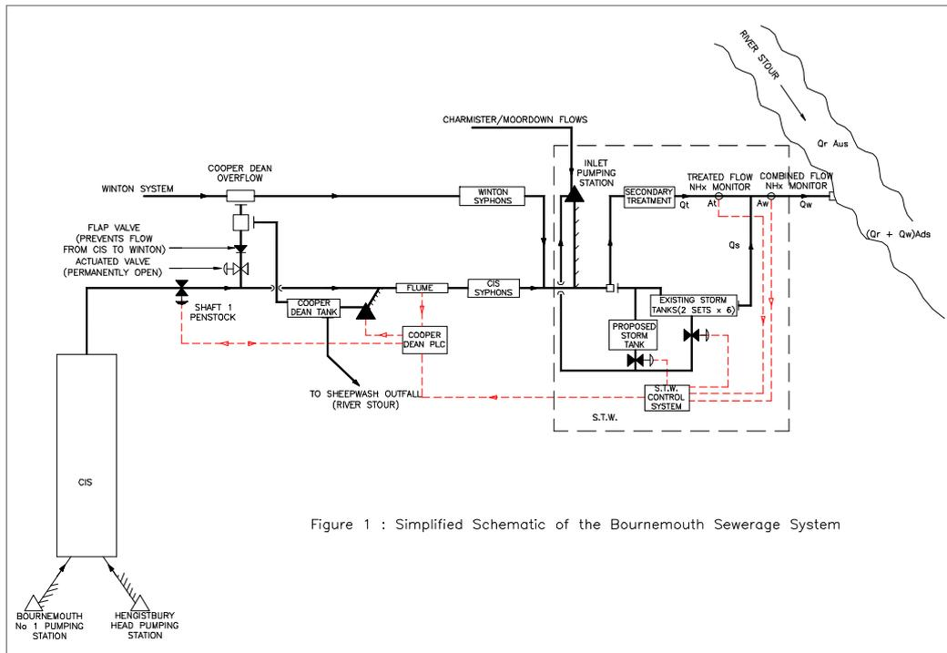
Figure 1 : Simplified Schematic of the Bournemouth Sewerage System
