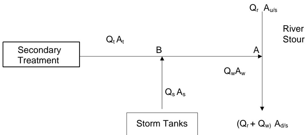
(The controller assumes that  $Q_w$  is equal to the flow into the STW when the storm tanks are full – negligible flow losses through the STW)
