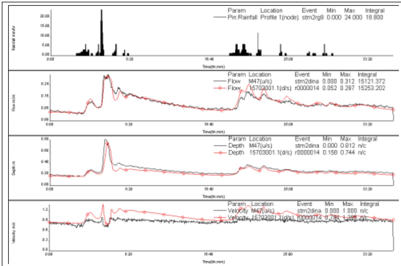
**Figure 2- Model verification plot showing wet weather infiltration**
