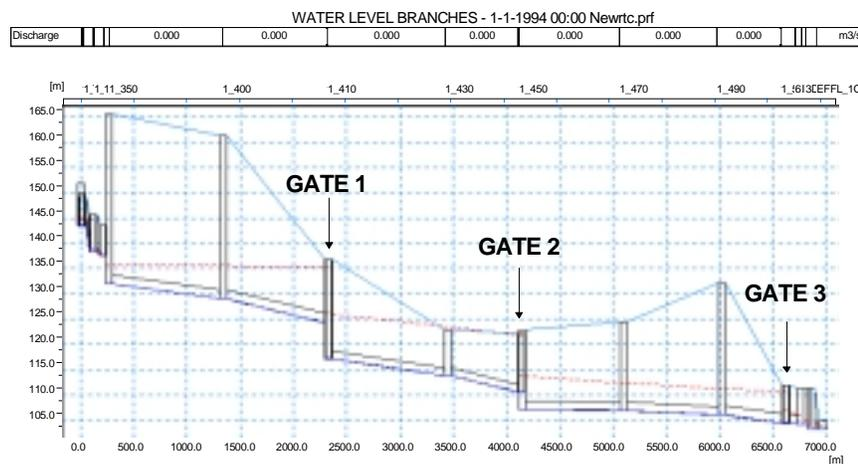
Figure 2: Long section of ODIS showing Gates 1, 2 and 3
