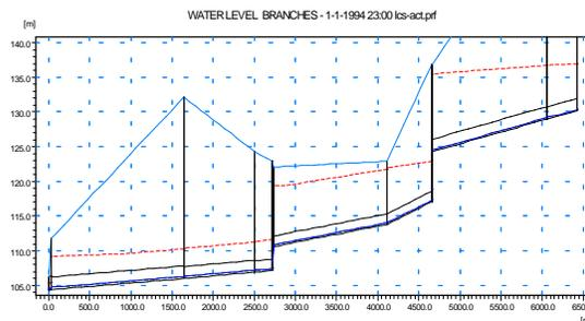
**Figure 6 Longitudinal profile through ODIS (controlled flow)**
