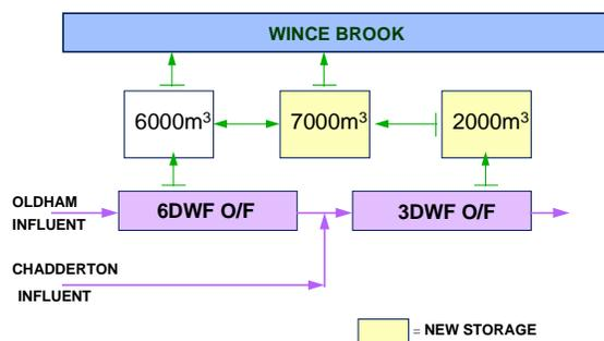
**Figure 4 Schematic of the planned storage at Oldham WwTW**
