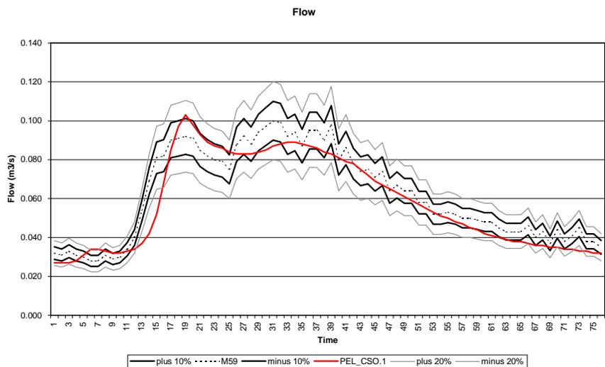
The envelope boundaries can easily be calculated by using a spreadsheet program. The graphs can easily be produced using the spreadsheet program or by exporting back to Hydroworks for plotting. It is also possible to fill in a sensible envelope boundary for odd times when the flow monitor is ragged or loses velocity data for a short period.
