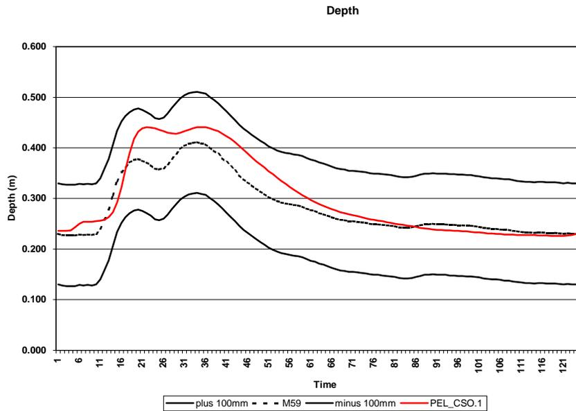
The observed data is plotted with the  $\pm 100\text{mm}$  limits either side and the simulated hydrograph is then plotted against these. If the simulated results stay within the envelope then the depth verification can be considered satisfactory.
