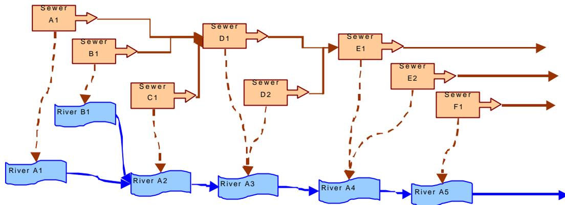
**Figure 4 Schematic of simplified sewer catchment model**
