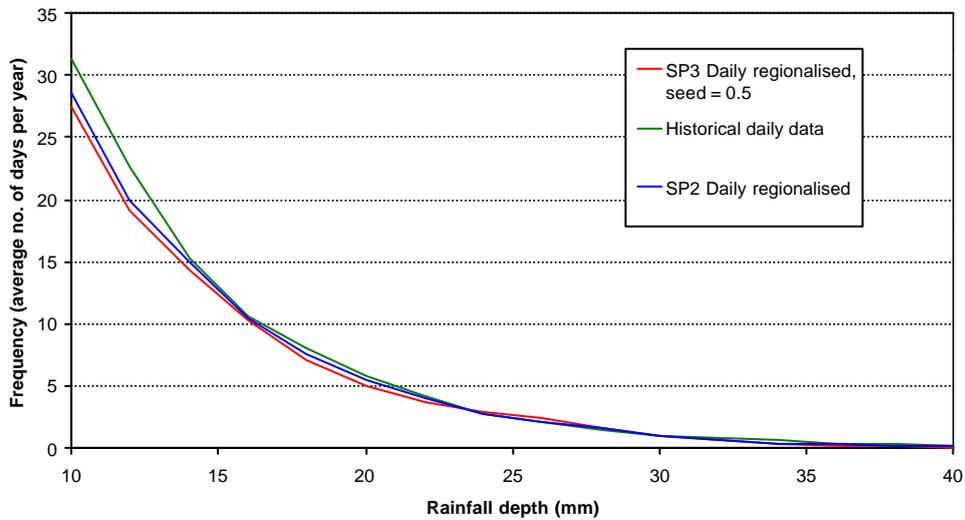
Figure 2 Examples of threshold analysis of daily totals of simulated rainfall
