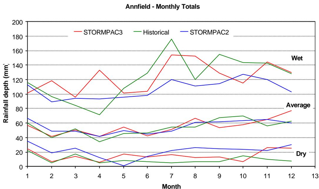
**Figure 3 A comparison of simulated and historic monthly totals at one test site**
