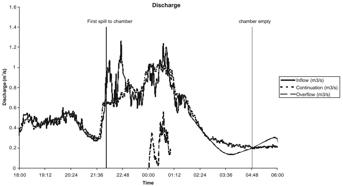
**Figure 3: Flow and quality data in off-line chamber**
