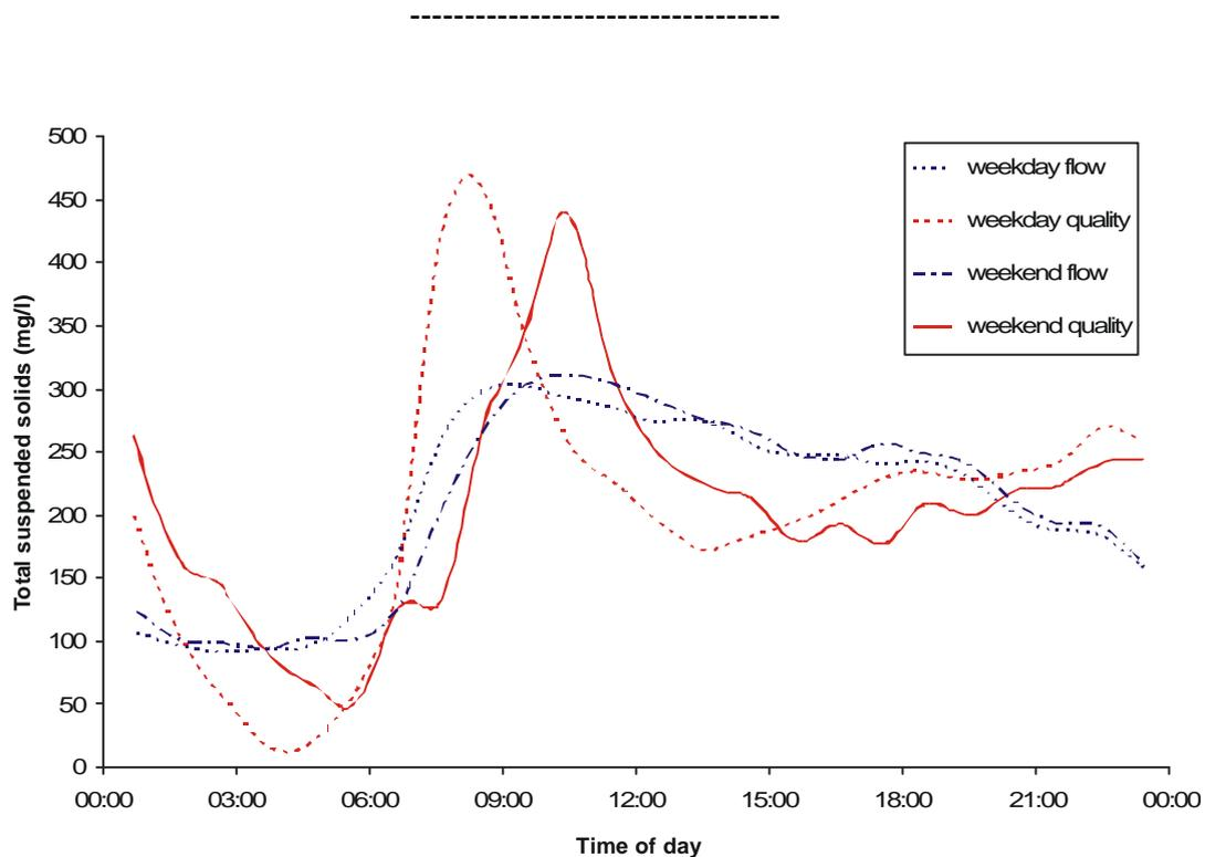
Figure 1: Typical diurnal patterns of the quality of dry weather flow
