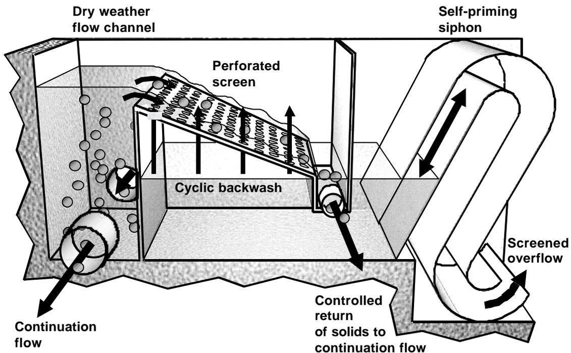
Figure 1 Schematic Representation of the Hydro-Jet Screen™
