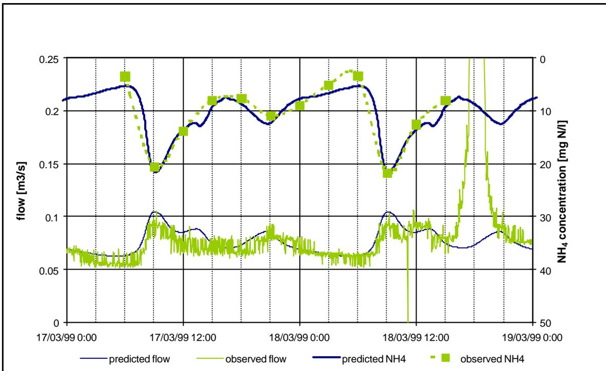
Figure 4 Wezembeek Oppem – Dry Weather Flow 17-03-99 – Predicted and observed flow and NH<sub>4</sub> concentration
