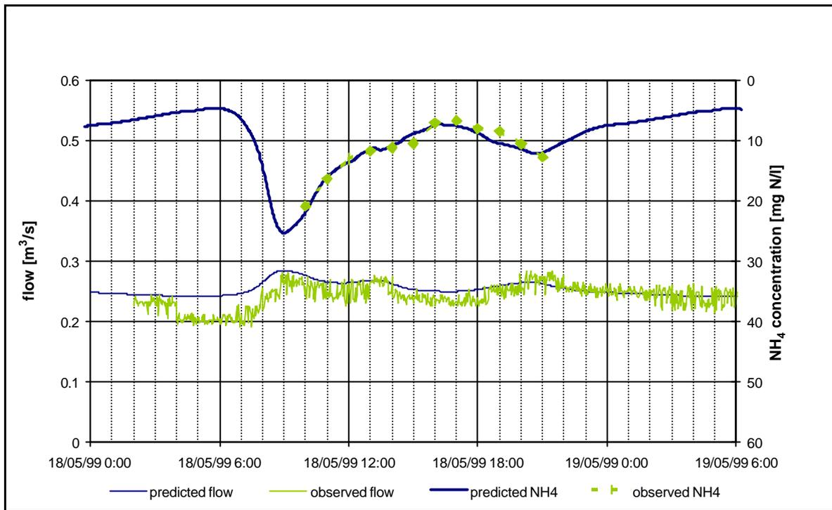
**Figure 7** Wezembeek Oppem – Storm of 18/05/99 – Predicted and observed flow and NH<sub>4</sub> concentration
