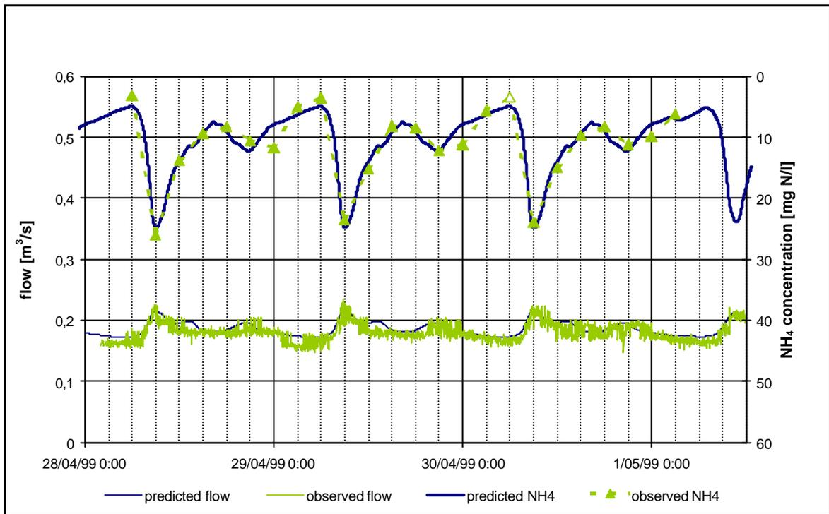
**Figure 5 Wezembeek Oppem – Dry Weather Flow 28/04/99 – Predicted and observed flow and NH<sub>4</sub> concentration**
