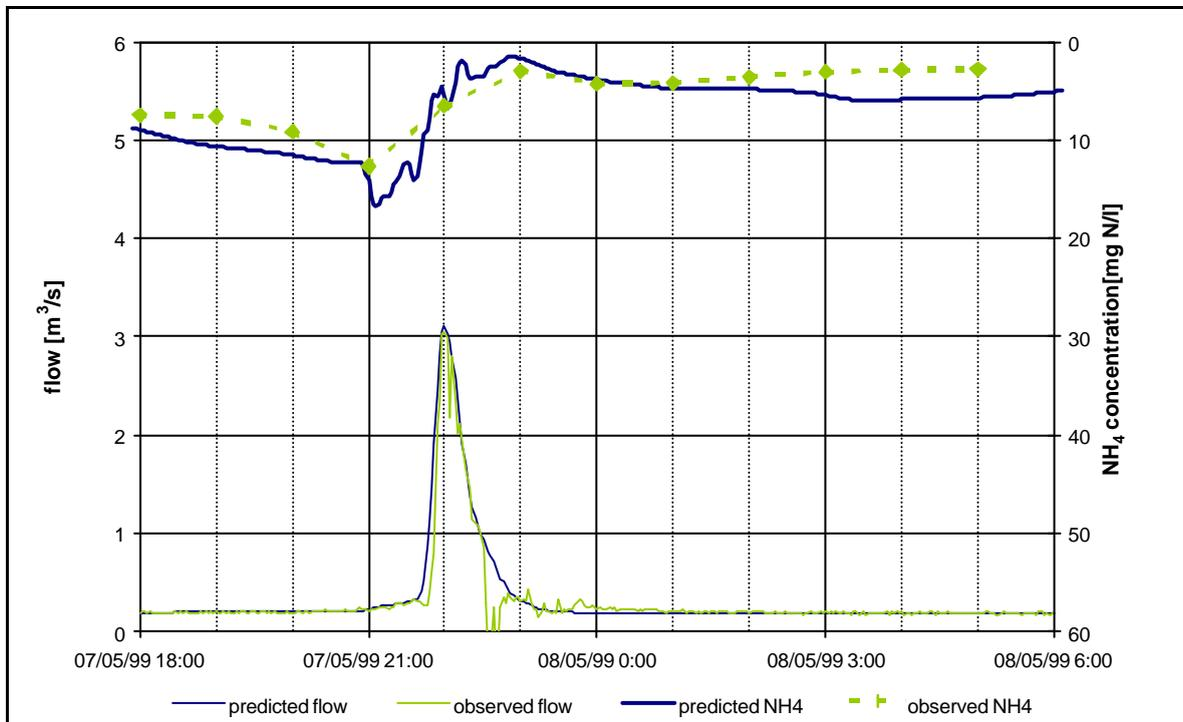
**Figure 6 Wezembeek Oppem – Storm of 07/05/99 – Predicted and observed flow and NH<sub>4</sub> concentration**
