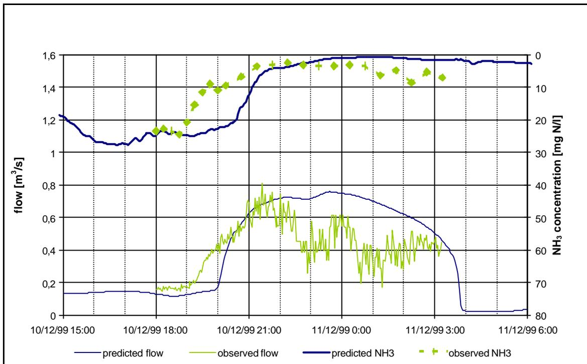
**Figure 10** Burslem Tunstall – Storm of 10/12/99 – Predicted and observed flow and NH<sub>4</sub> concentration
