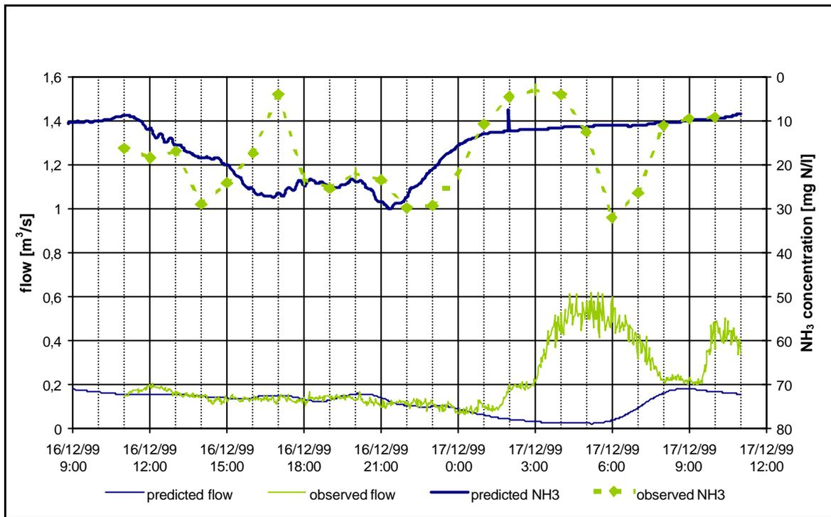
**Figure 9** Burslem Tunstall – Dry Weather Flow 16/12/99 – Predicted and observed flow and NH<sub>4</sub> concentration
