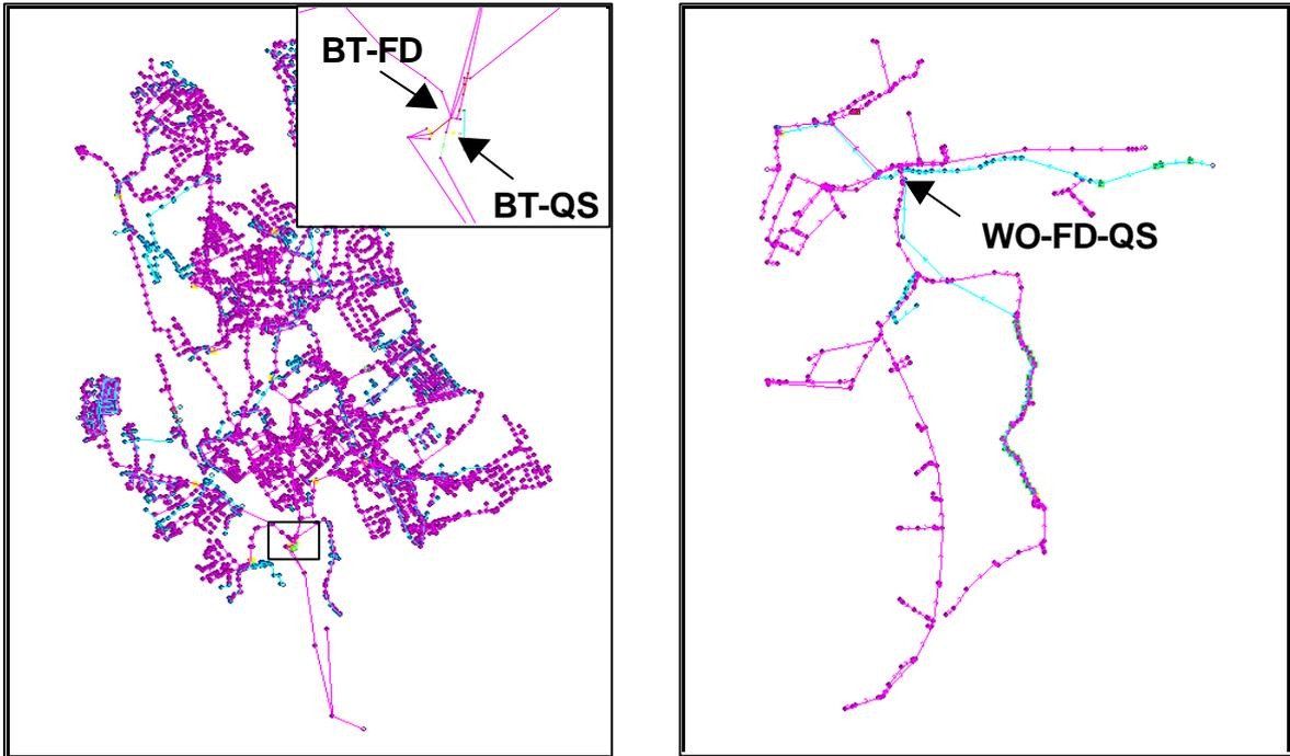
**Figure 1** The Burslem Tunstall catchment (left) and the Wezembeek Oppem (right) including monitoring sites of flow data (FD) and quality sampling (QS)
