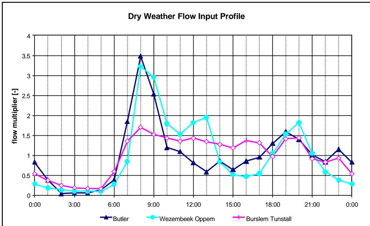
**Figure 2** Domestic wastewater input profile
