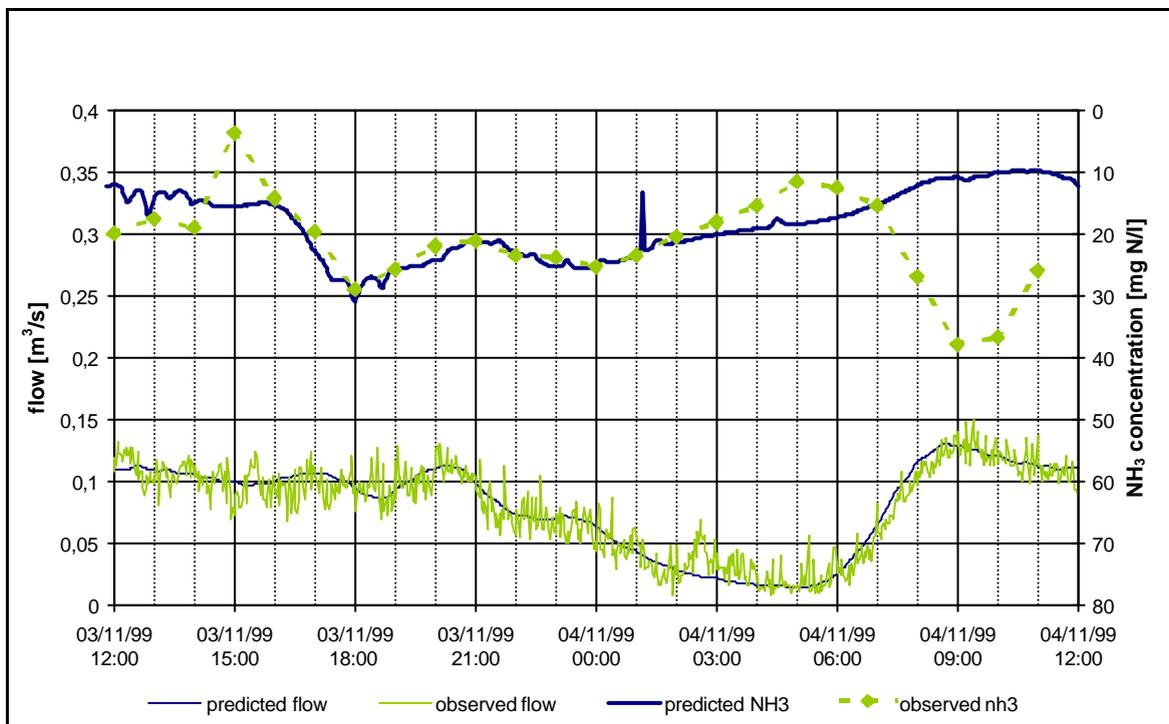
**Figure 8** Burslem Tunstall – Dry Weather Flow 03/11/99 – Predicted and observed flow and NH<sub>3</sub> concentration
