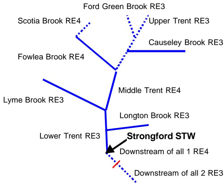
Figure 4. EA River Quality Objectives used in the SIMPOL model. Reaches failing RQOs shown thus: .....
