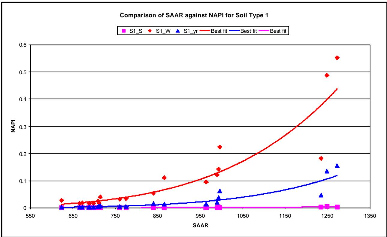
Figure 3a Comparison of SAAR against median NAPI – Soil 1
