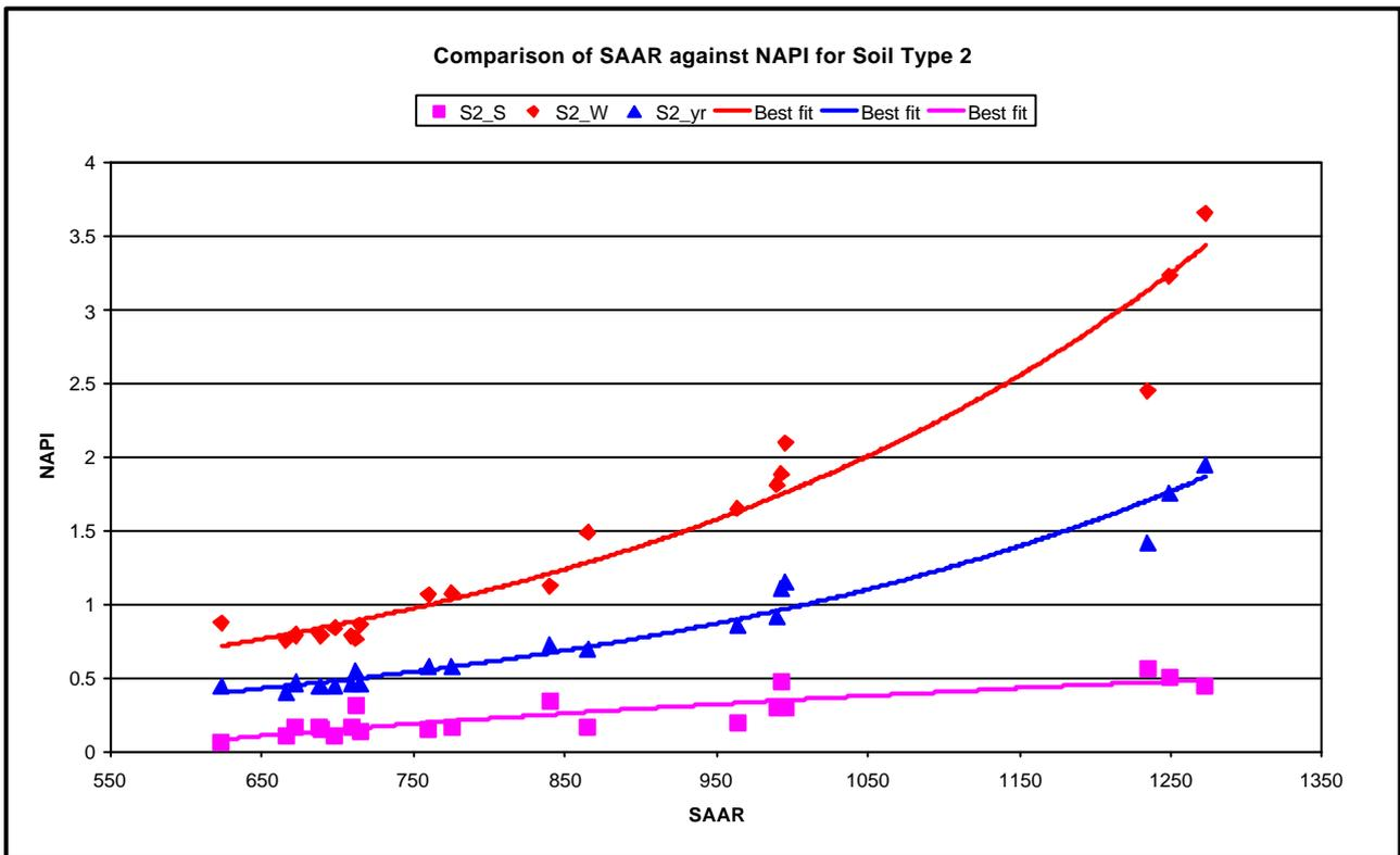
Figure 3b Comparison of SAAR against median NAPI – Soil 2
