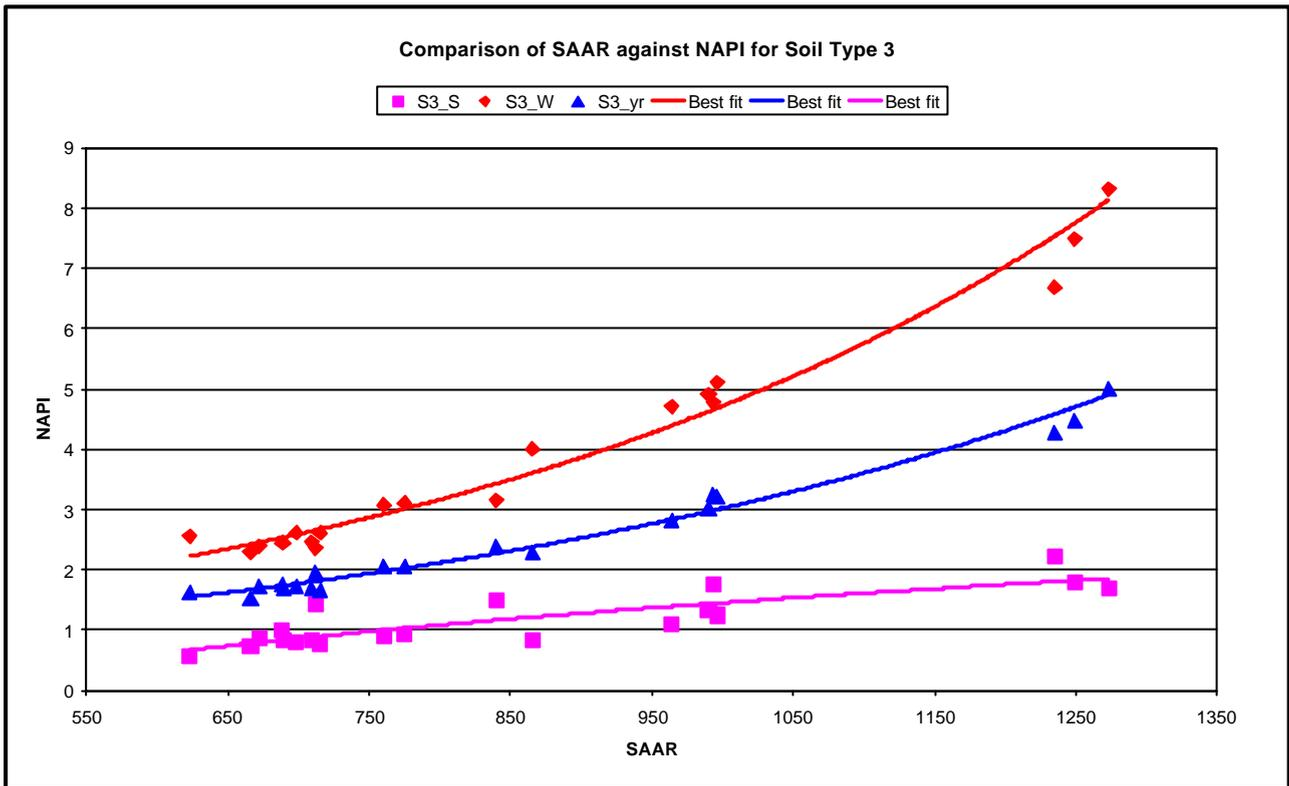
Figure 3c Comparison of SAAR against median NAPI – Soil 3
