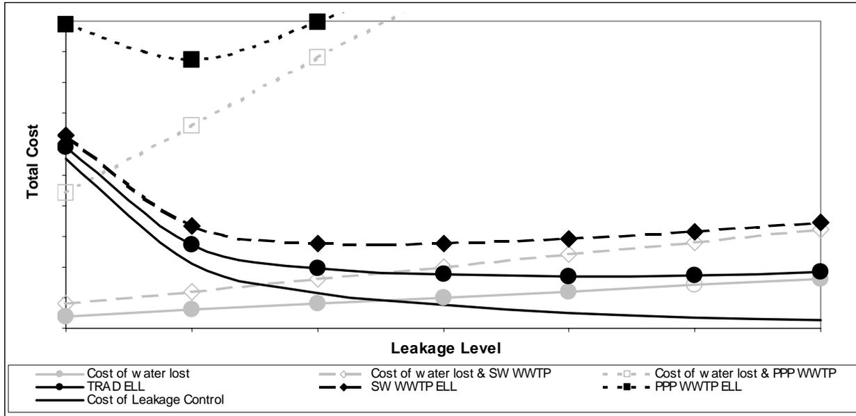
**Figure 3 - Effect on calculation of economic level of leakage**
