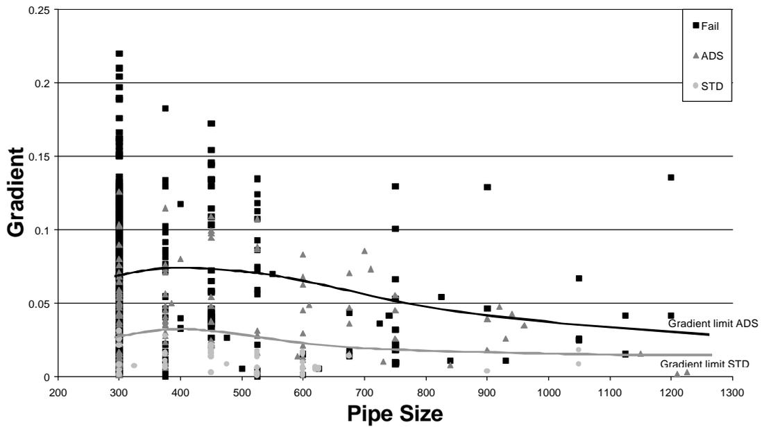
**Fig. 3: Graph showing influence of gradient and pipe size on flow monitoring performance and recommended maximum gradients for flow monitoring, based on Event 22.**
