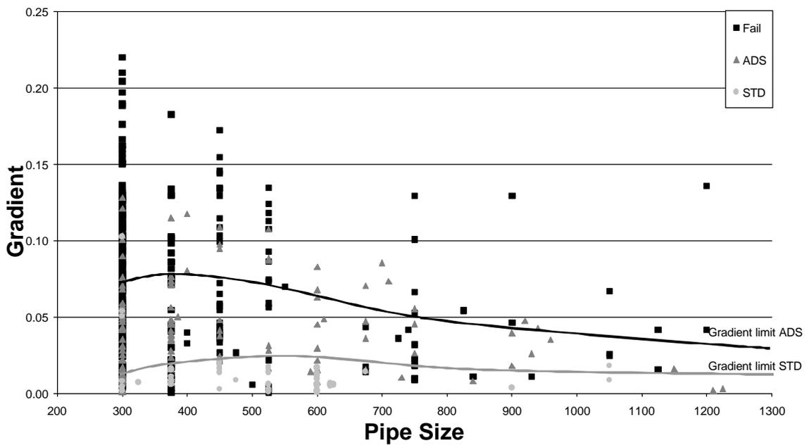
**Fig. 4: Graph showing influence of gradient and pipe size on flow monitoring performance and recommended maximum gradients for flow monitoring, based on Event 31.**
