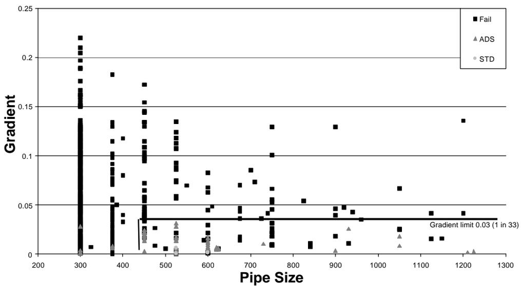
**Fig.2: Graph showing the influence of gradient and pipe size on flow monitoring performance and recommended maximum gradients for monitoring in Dry Weather Flow Conditions**
