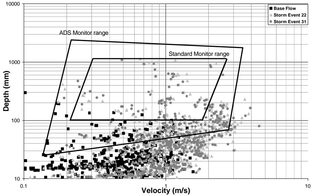
**Fig. 1: Polygon comparing 75 % depth and velocity for each pipe, with the range of accuracy of flow monitors.**
