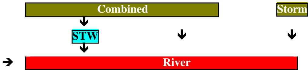
The upstream river boundary is normally represented by a random selection from a statistical distribution for both flow and pollution. However it is possible to model the flow using a rainfall runoff model. A model representation of the pollution concentration is also possible but this would require a complex river model and is beyond the scope of this paper.
