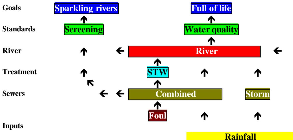
Each of the components of rainfall, foul flow, sewers, treatment works and river needs to be represented by some form of model and there are often a variety of models of
