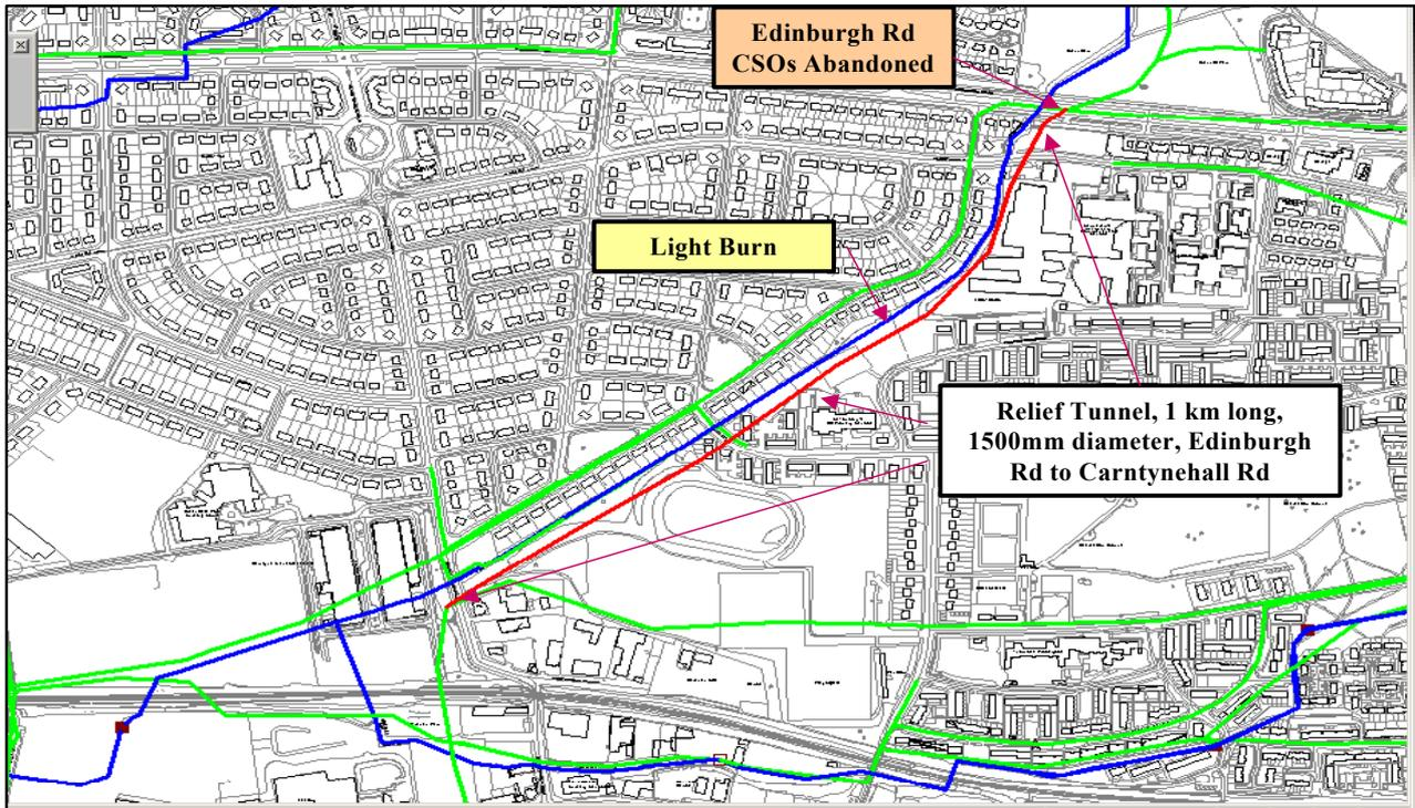
Figure 4 – Interceptor Tunnel Scheme
