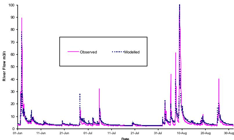
Each river reach has its own subcatchment, each of which can have different applied rainfall series – this allows spatial patterns in rainfall to be taken into account. An example of river flows generated by SIMPOL3 are shown in Figure 3.
