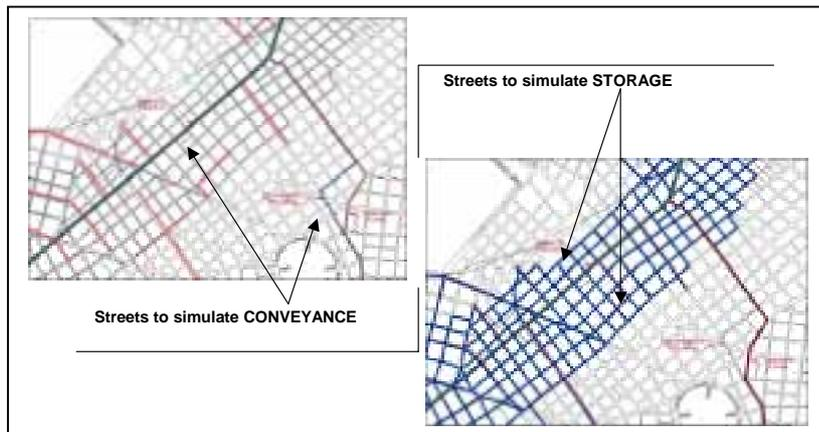
**Figure 4:** Schematic representation of conveyance and storage in the overland flow system.
