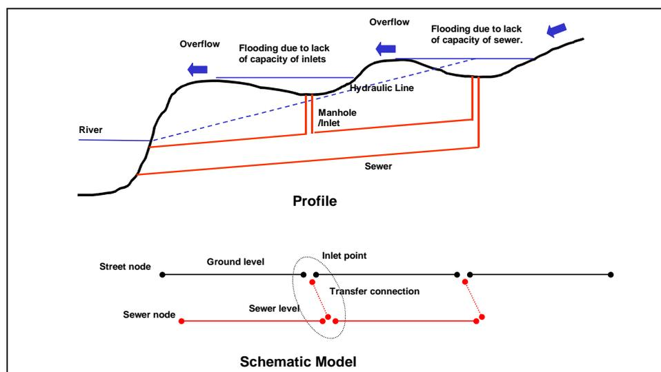
**Figure3: Schematic representation of the two flooding situations.**
