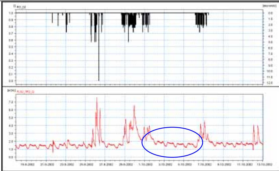
**Graph 1: An example of Slow Runoff Component (SRC) observed at WWTP inlet**
