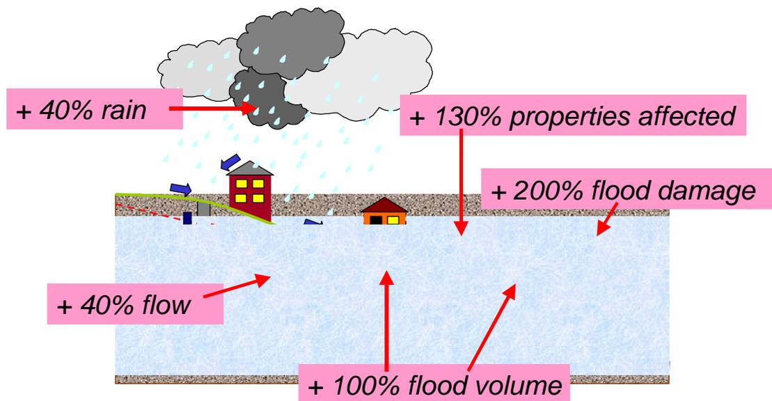
**Figure 1 The potential impacts as a result of climate change on the urban drainage system.**
