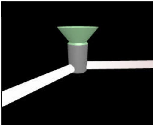
Figure 5 – Manhole with no over land flood channel applied. The shaft and chamber plan area are both 1.5m<sup>2</sup>.<sup>†</sup>
