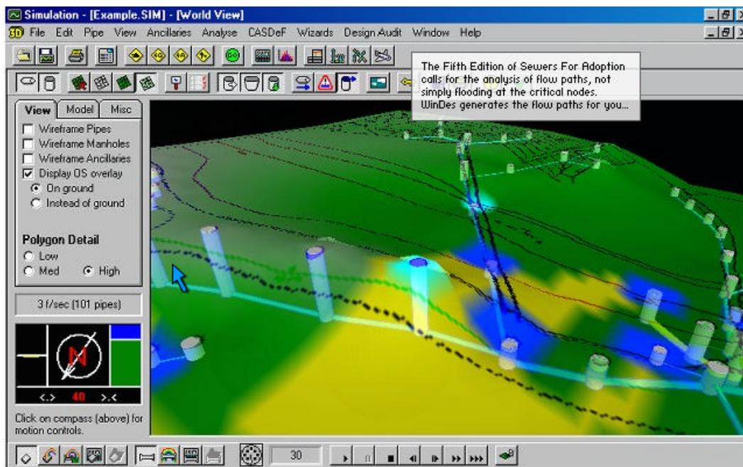
Figure 4 - WinDes 3D sewer modelling for design purposes, (source – Micro Drainage's WinDes 'Future Engineering' CD).
