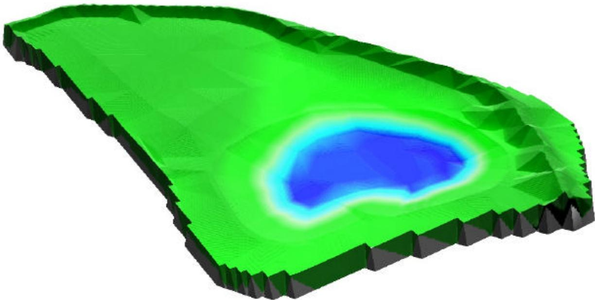
*Figure 3 - 3D Thematic of the Rockfield Storage Pond, Monmouth. Map is based upon land survey data undertaken as part of the Wonastow Brook Flood Alleviation Scheme.*
