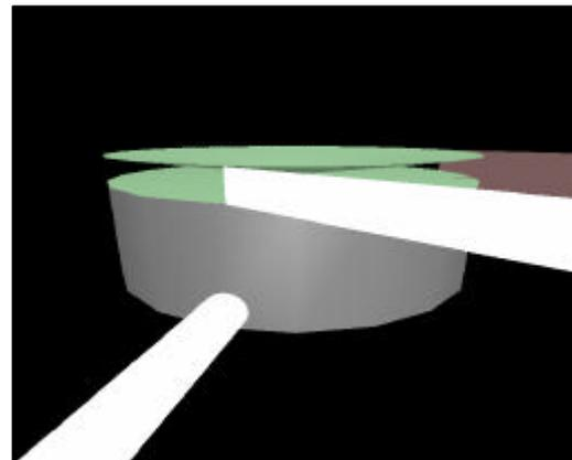
Figure 6 – Manhole with an overland flood channel where the invert level is set to the cover level of the manhole. The shaft and chamber plan both increase to 35.9m<sup>2</sup>.<sup>†</sup>
