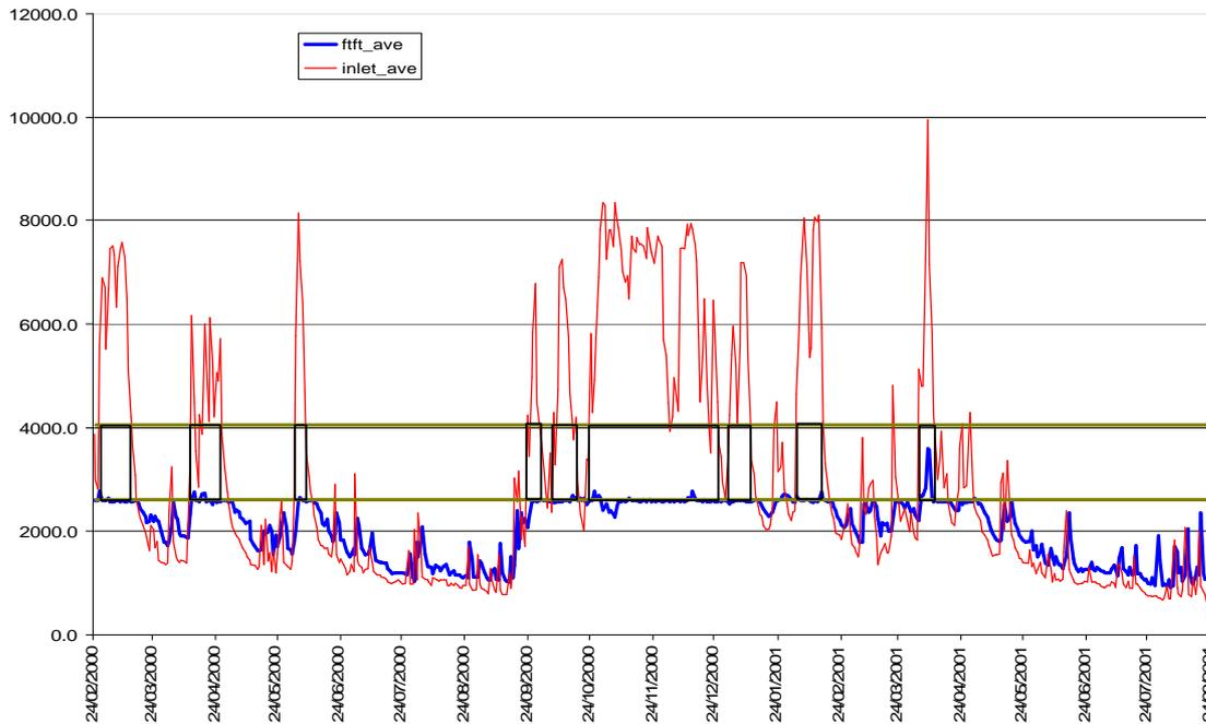
**Figure 1: Impact of Increased FFT on Storm Tank Spill Frequency**
