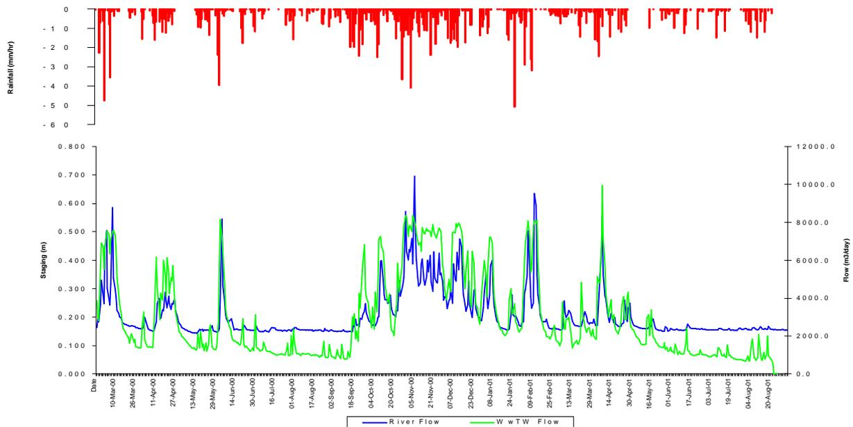
**Figure 2 Correlation between River Flow, Inlet Works Flow and Rainfall at Ripponden**
