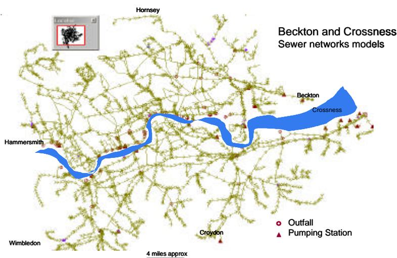
Thames Water has InfoWorks network models covering the major sewerage catchments of London. The Beckton and Crossness catchment area (Martin, 1995) is modelled with all main sewers and diversion and bifurcation structures. This was completed in the mid 1990s and calibrated with the best available
