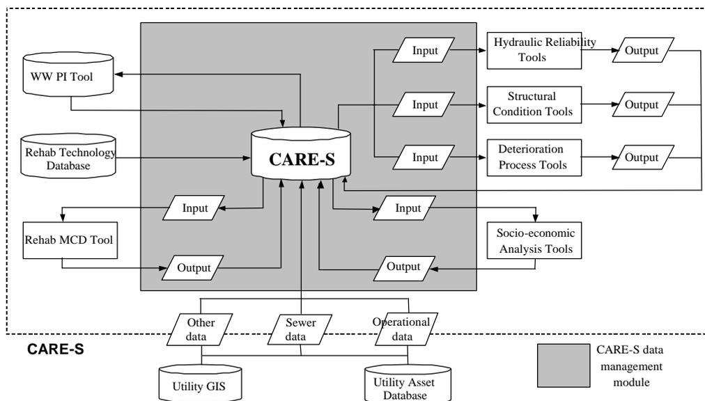
**Figure 1.** The general architecture of the CARE-S Sewer Rehab Manager
