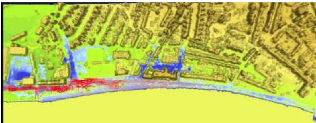
Figure 5 Example of Results from Overland Flow Due to Overtopping Simulation a) Two-Dimensional Representation and b) Three-Dimensional Representation Showing Depths (Blue) and Velocity Vectors (Red)
