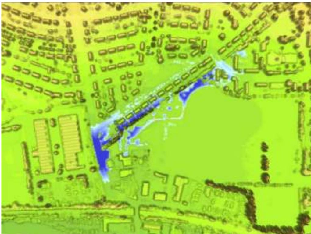
Figure 7 Example of Results from Overland Flow Due to Sewer Overflow Simulation a) Two-Dimensional Representation and b) Three-Dimensional Representation
