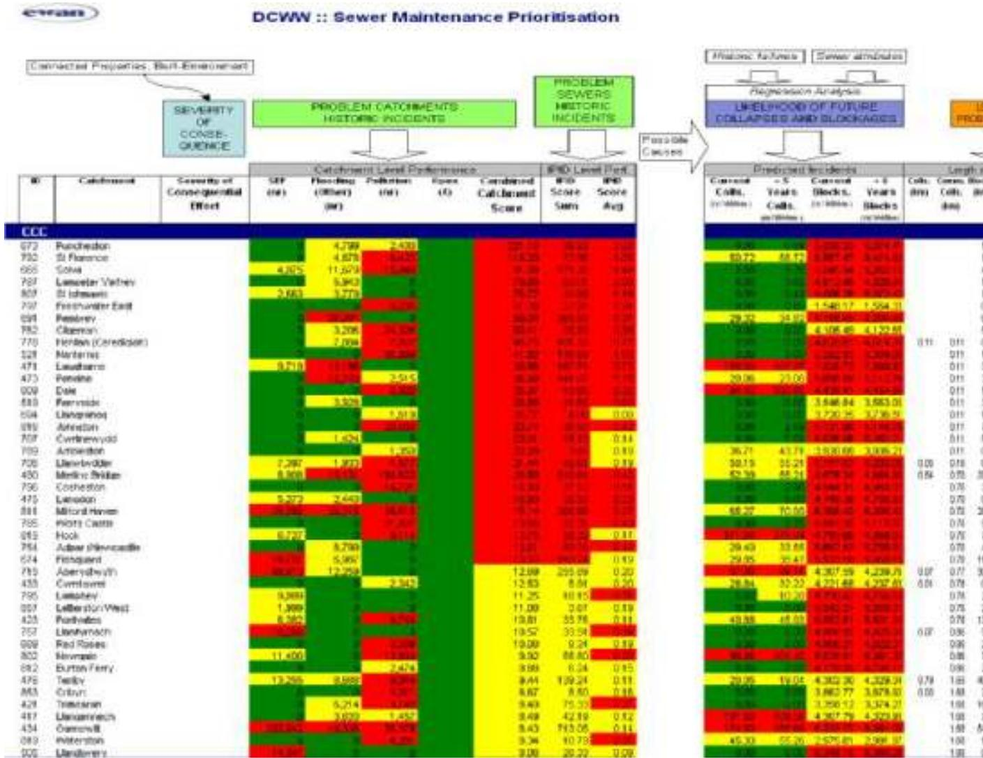
Figure 3.5 Illustrative results for DCWW risk-based sewer maintenance prioritisation
