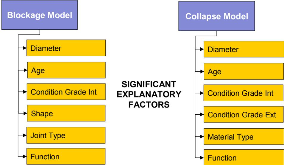
**Figure 3.4 Significant explanatory factors of asset performance failures**
