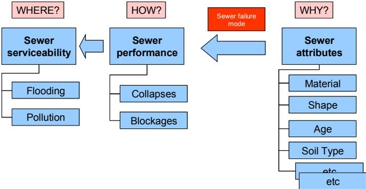
Figure 3.1 illustrates the concept of separating asset service, asset performance and explanatory factors.
