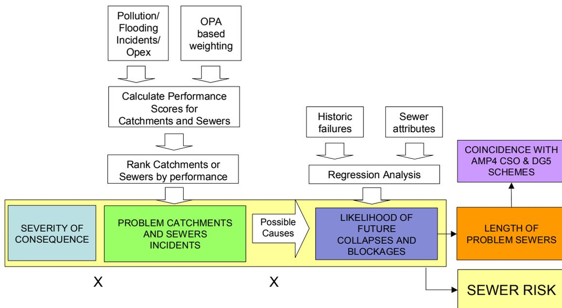
Figure 3.3 Risk based prioritisation of sewerage maintenance
