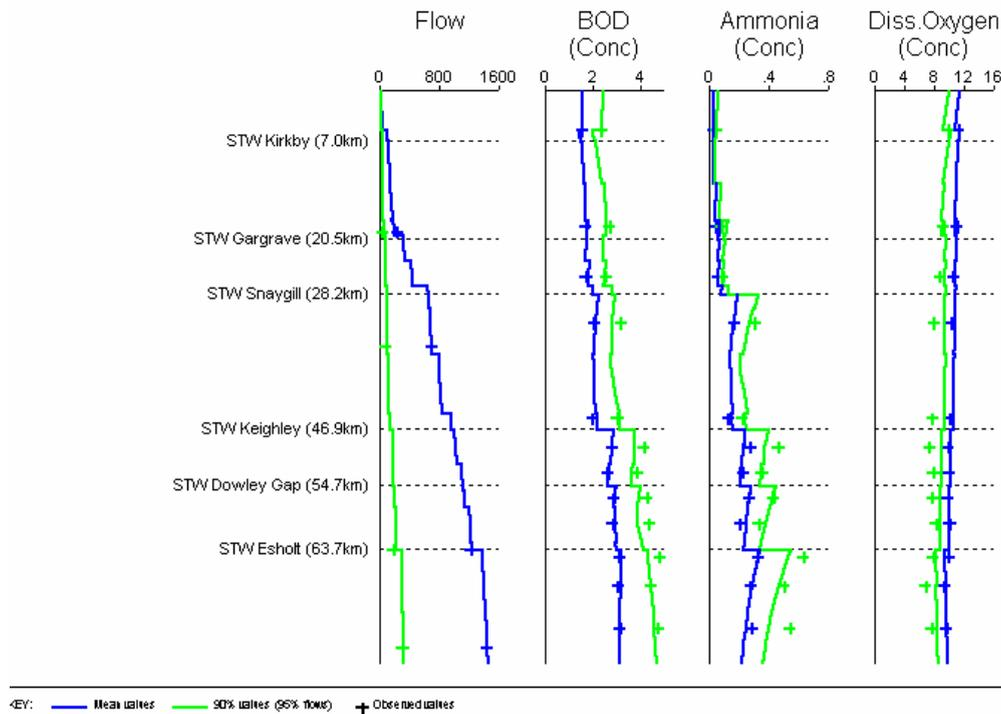
**Figure 4 River Aire Manual Calibration for Flow, BOD, Ammonia and DO**
