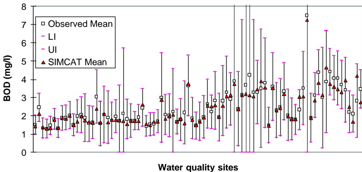
**Figure 3 Manual calibration results for BOD**
