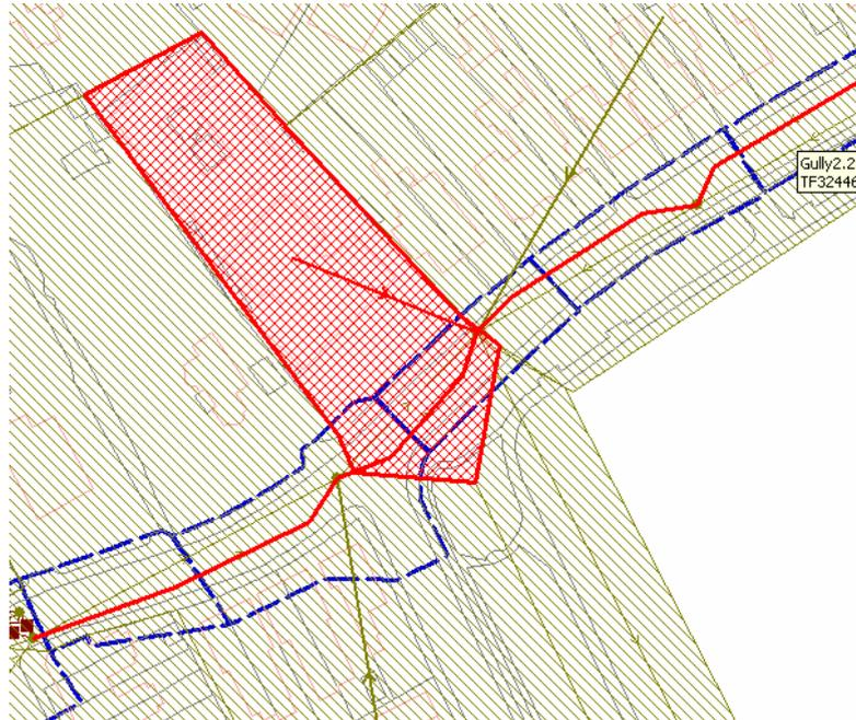
Figure 3: The difference between subcatchments and floodable areas (blue polygons), with dummy channels highlighted
