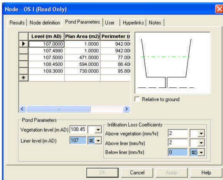
The small plan area and large perimeter are used to represent the loss through the flat base of the pond.
