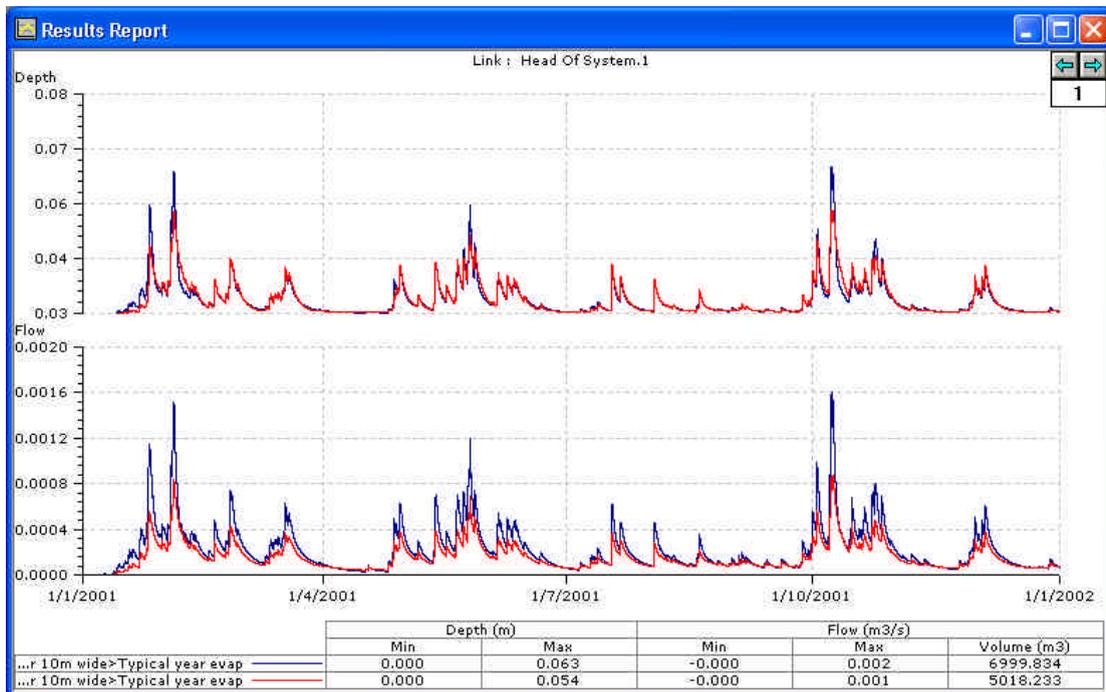
From the graphs it can be seen that differing k values have a greater impact during large events. As expected, reducing the Darcy k value, reduces the conductivity of the trench and therefore causes the overflow ditch to operate more frequently, as presented in the table below.
