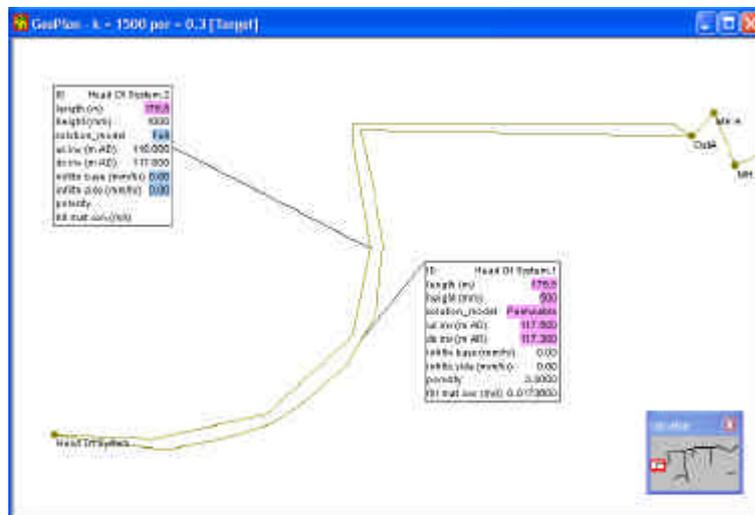
One of the main limitations in this representation is that the trench and the ditch are only connected at the top and bottom, whereas in reality there would be continuous cross
