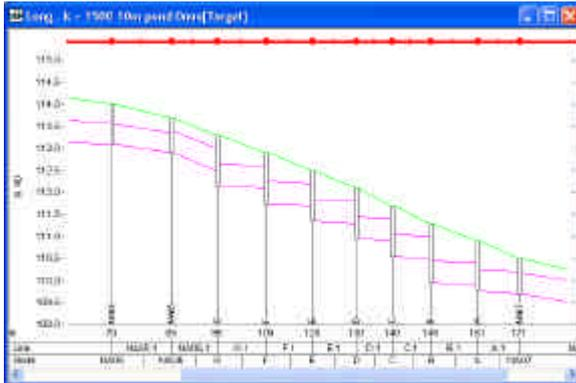
The cascade was modelled as a series of short open channels, as shown in the adjacent figure. It was found that changing hydraulic roughness and even the geometry of the model had little effect on hydraulic performance within the cascade itself. The model results, whilst not being able to replicate the exact flow categories along the length of the cascade gave realistic results in terms of outflow depths and velocities.
