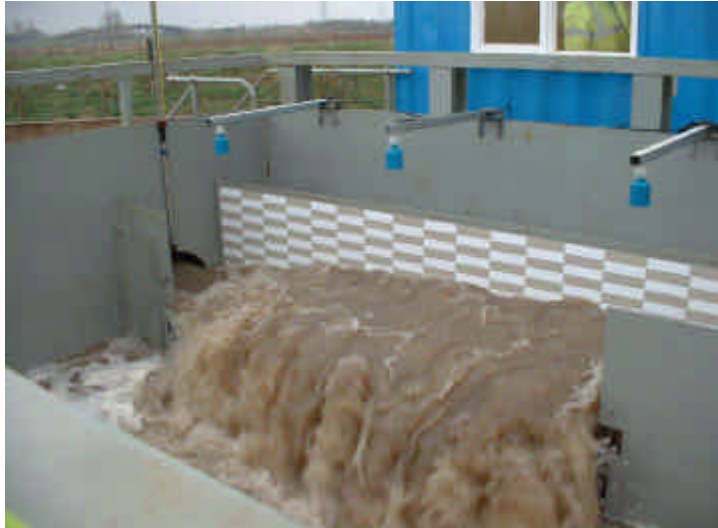
Figure 2. Side Weir CSO Under Test at High Flow showing the Formation of a Hydraulic Jump in the Weir (courtesy United Utilities )
