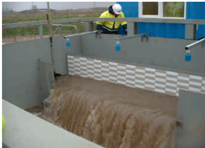
Figure 1. Side Weir CSO Under Test at Low Flow showing Rising Water Surface Profile (courtesy United Utilities)
