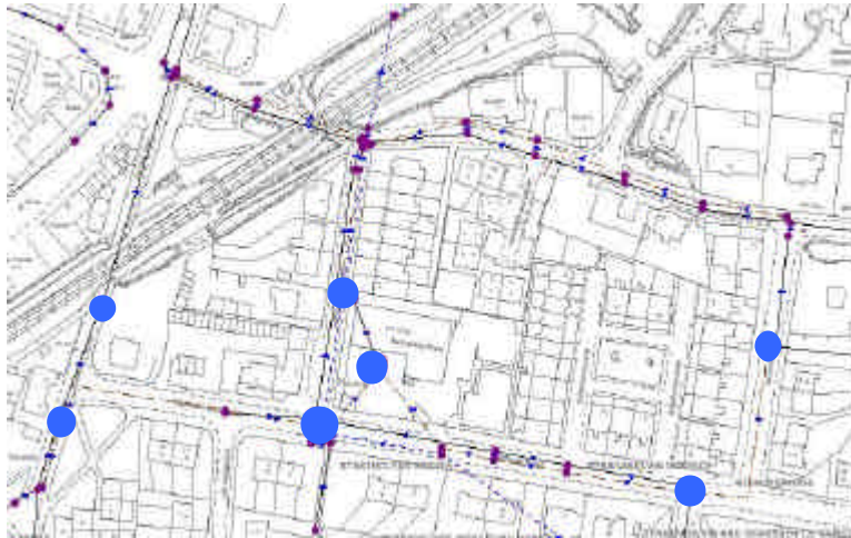
Figure 3. Flood Locations from Conventional Sewer Network Model. In this case the location of flooding was found to be significantly different from that reported at the time of the event
