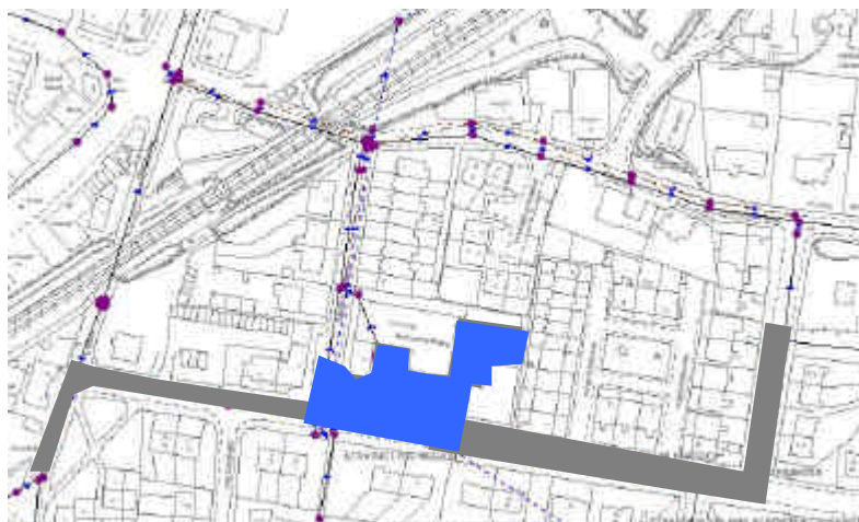
Figure 4. Improved Representation of Flood Location by Explicit Modelling of Above Ground Flood Pathways With the surface flood channels modelled the location and mechanism of flooding is correctly identified.
