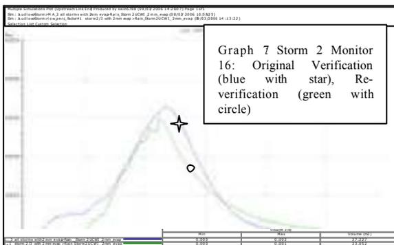
For the groundwater module the evaporation during the dry period has the additional effect of lowering the soil store depth. Thus, by the time the second verification event occurs the soil store depth is below the percolation threshold (the level at which infiltration to the sewer system occurs). As a result, the first part of the rainfall for the second event is taken up
