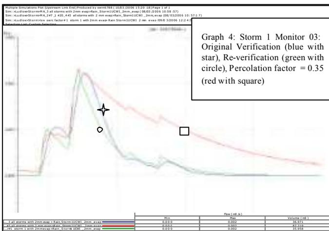
Storm one had an UCWI value of 167 and occurred within the first two weeks of the flow survey. Between storm one and storm two there was a period of approximately two months with relatively dry weather. Thus, when storm two occurred the UCWI value had declined to only 126. This has a different effect on the original
