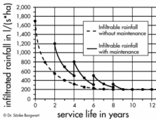
Much of the evidence indicates that a significant factor in whether a pavement clogs is the presence of adjacent landscaping. American, Japanese, French and German experience with permeable concrete block surfacing suggests that the design infiltration rate should be 10 per cent of the initial rate to allow for clogging over a 20 year life.
