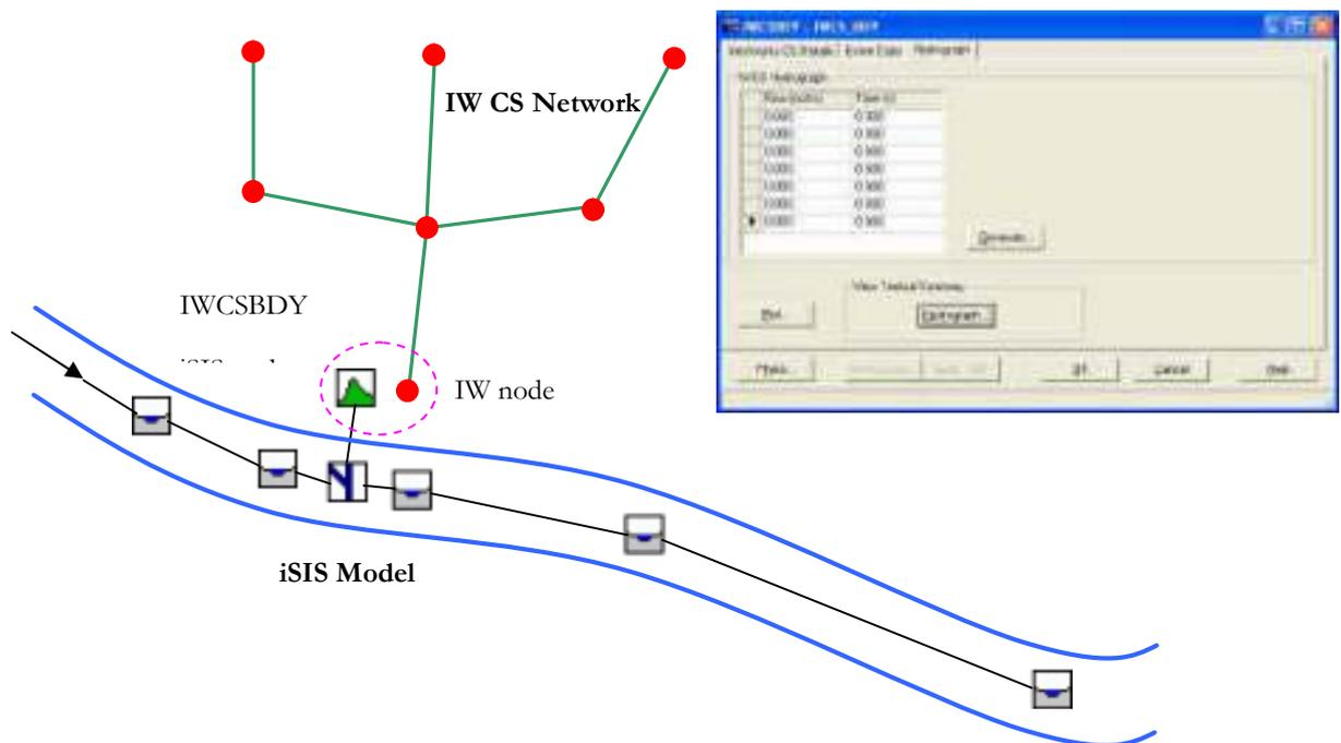
Figure 3: Static linking between ISIS and InforworksCS
