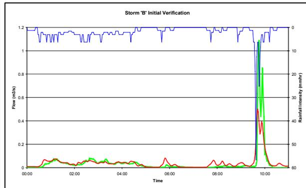
It was clear from these initial verification hydrographs that when there was higher intensity rainfall there was a considerably greater flow in the system which could only be caused by additional areas contributing runoff. Clearly in periods of lesser intensity these additional areas do not normally contribute runoff. It was only the storm with peak intensities in excess of 25mm/hr (or even higher) that caused these additional areas to contribute runoff.
