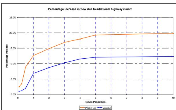
Different versions of the model can be run with and without the highway runoff component so that the differences which are attributable to the additional highway runoff can easily be determined.
