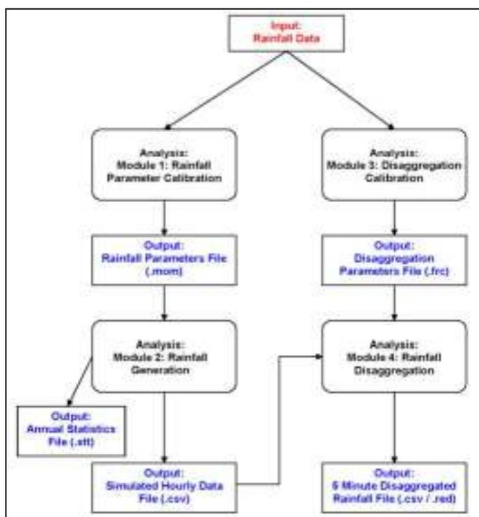
Figure 1: TERSim Program Flow Chart (extract from TERSim User Guide)
