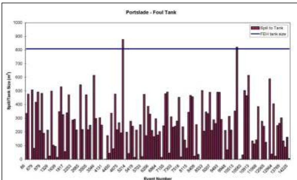
Figure 2 - Predicted spills to Combined tank using TSRSim Rainfall
