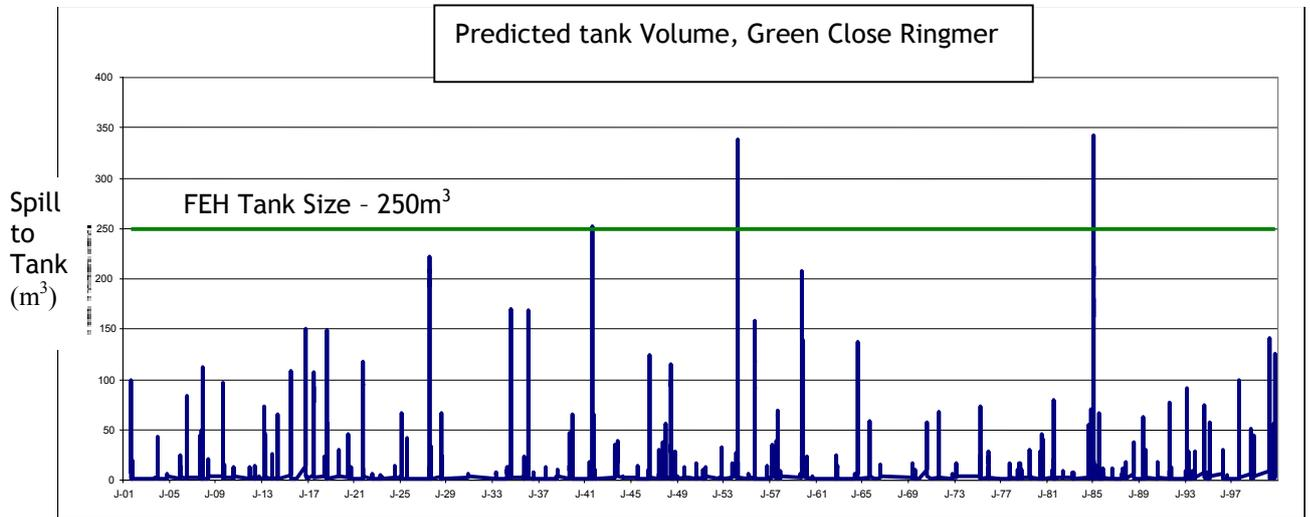
Figure 3 - Ranked spills to storage tank and FEH storm tank size, Green Close Ringmer
