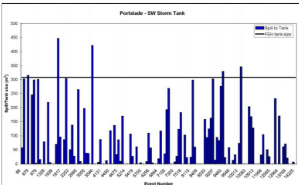
Figure 3 - Predicted spills to Surface Water tank using TSRSim rainfall
