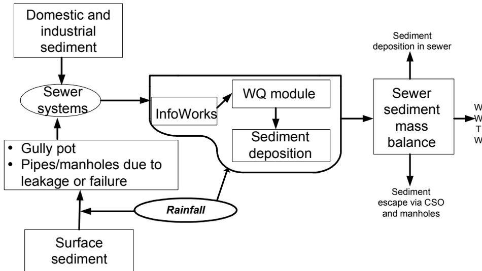
Figure 2 - Overall conceptual approach to sewer sediment modelling using *InfoWorks CS*
