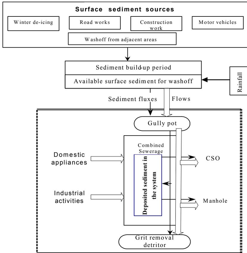
Figure 1 - Flow diagram of sediment fluxes in drainage systems (Gouda, 2004)
