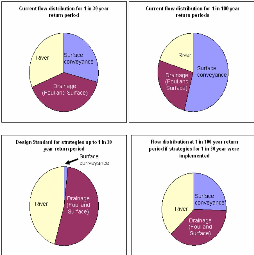
**Figure 4. Current and Potential Contributions of the Different Drainage Modes in North Brent**
