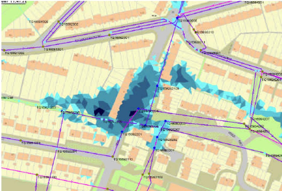
**Figure 3. Integrated Model with Full Dynamic Interaction between Sewerage Systems, the Watercourse and Surface 2D Flooding, using InfoWorks 2D.**
