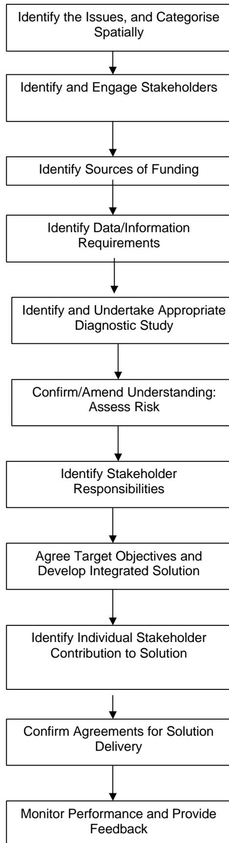
**Figure 2. Flow Chart for Integrated Urban Drainage (from Defra IUD Pilots Scoping Study (Balmforth et al, 2006.1))**
