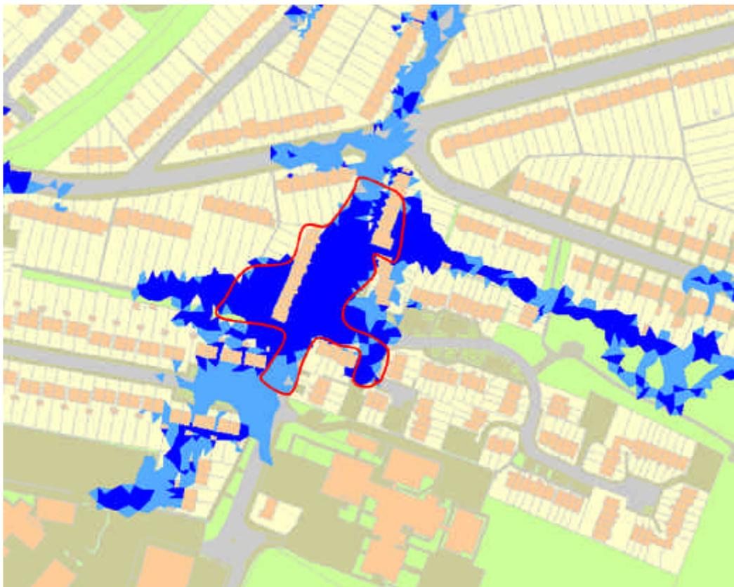
**Figure 6** Catchment 1, detailed sub catchment area, coupled sewer and 2D overland flow routing for event of July 2007. The figure indicates the known flooding from video evidence as a thin line. The simulation is shown in a dark shading to represent predicted depths above 50mm and lighter colour is above 10mm.
