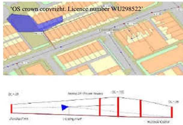
Figure 7. Predicted flooding location with lateral representation.
